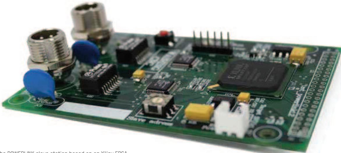
The POWERLINK slave station based on an Xilinx FPGA.
