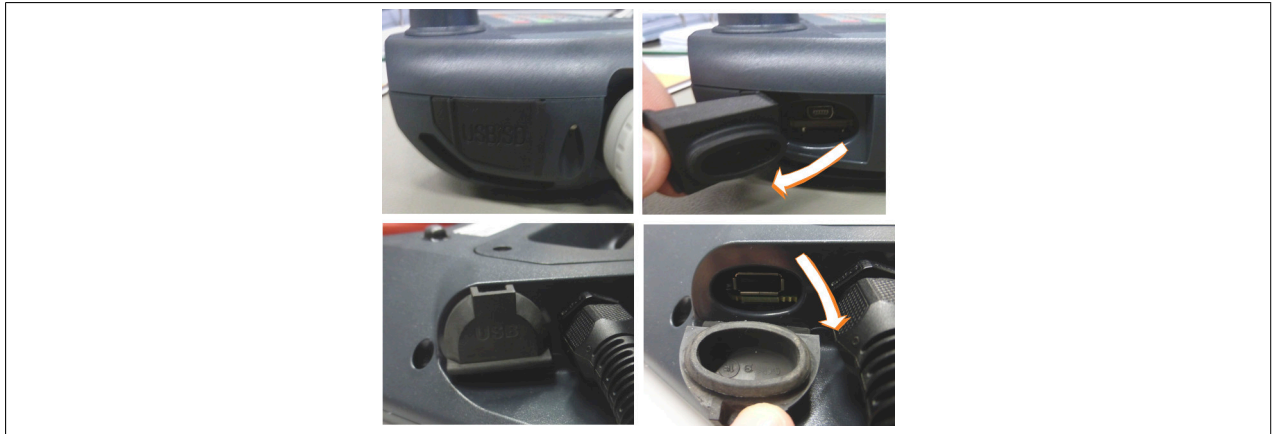
Figure 28: USB interface - Opening the protective cover
