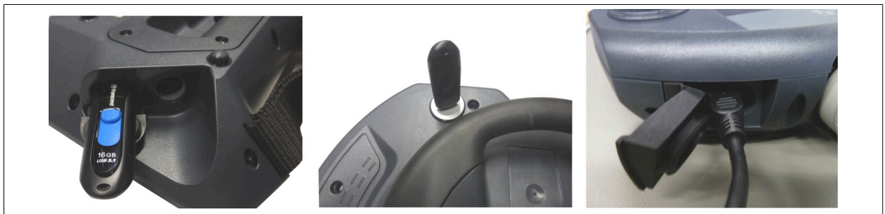
Figure 30: USB interface - Connecting the USB device
