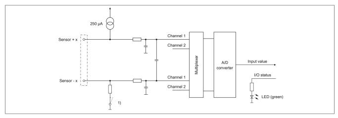
1) Switch is closed for 2-wire connections.
