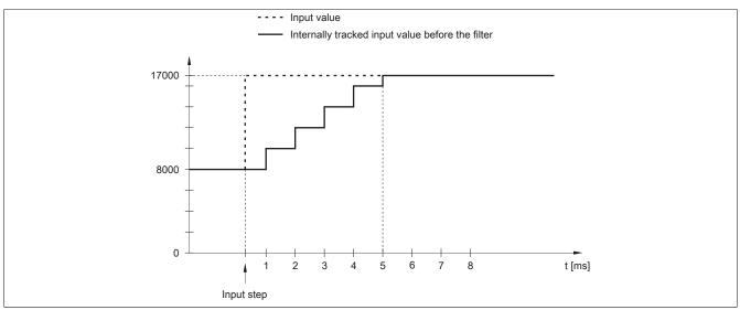
Figure 1: Tracked input value for input step
