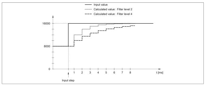
Figure 3: Calculated value during input step
