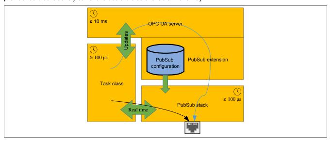
Each PubSub frame can be sent with its own cycle time and a time offset within the cycle. The network must provide appropriate mechanisms to also guarantee these hard real-time requirements on the receiver side of the network.
