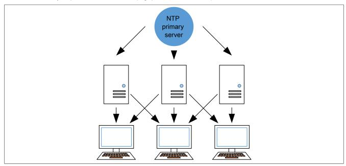
NTP is not suitable for industrial real-time Ethernet with accuracy requirements in the microsecond and sub-microsecond range, however, so most technologies use their own mechanisms for time synchronization. POWER-LINK, for example, uses the first frame in the cycle (SoC) that is sent by the master at highly precise, equidistant times to synchronize the stations. In other technologies (e.g. PROFINET, CIP Sync with EtherNet/IP), IEEE 1588 is used.
