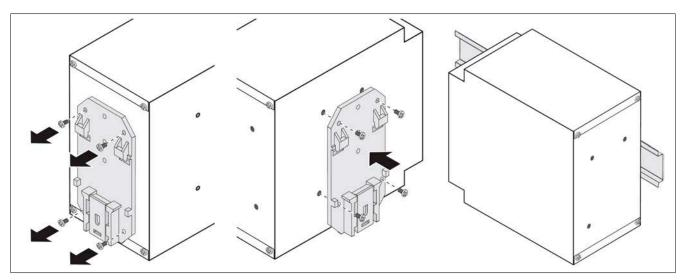
Wide installation can be achieved by mounting the device at a right-angle to the DIN rail. Mount the DIN rail adapter (UTA 107) as illustrated in the figure. No additional mounting material is required.
