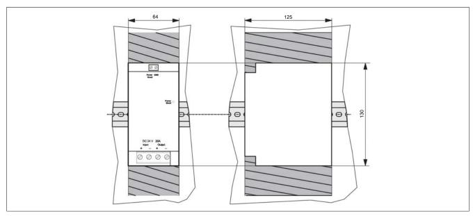
Narrow installation: Installation depth 125 mm + DIN rail (state at delivery)
