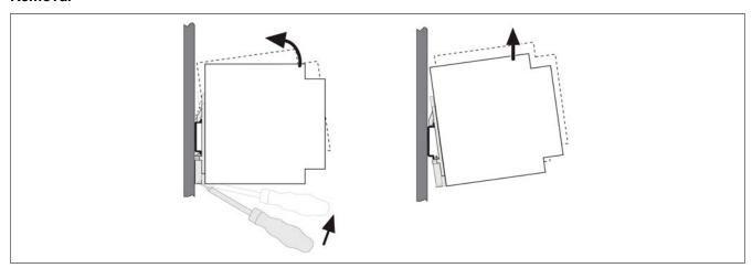
Pull the snap lever open with the aid of a screwdriver and slide the module out at the **lower edge** of the DIN rail.
