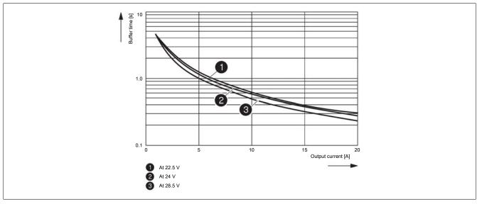
The connected devices can be divided into buffered and unbuffered loads using the isolated input This extends the buffer time, which depends on the output current. If only critical devices are protected using fuses, smaller battery modules can be used that save money and space in the control cabinet. In addition, the isolated input protects the connected devices against errors in the internal network.
