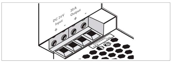
All loads that, in the event of a failure of the supply voltage, are to be supplied with power stored in the buffer module ("Buffered Load") are connected to the "+" and "-" of the DC output. We recommend that all other loads not requiring buffering in the event of a failure of the supply voltage ("Unbuffered Load") should be connected parallel to the power supply unit. This extends the buffer time, as it depends on the output current.
