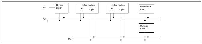
The buffer module is connected at the output of the power supply via the "+" and "-" screw connections of the 24 VDC input (4-pin connection). The output is decoupled from the input by means of the internal diode. The stored power is only delivered at the output.
