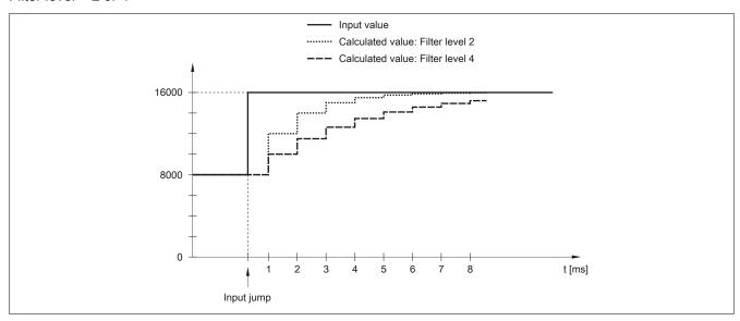
Figure 3: Calculated value during input jump
