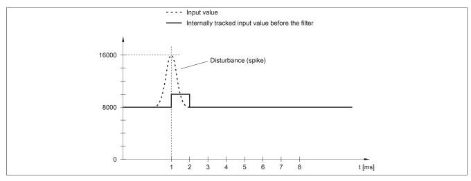
Figure 2: Adjusted input value for disturbance
