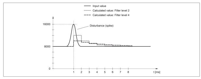
Figure 4: Calculated value during disturbance
