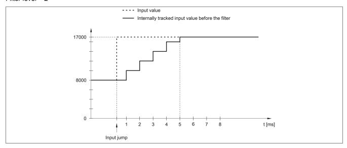
Figure 1: Tracked input value for input jump
