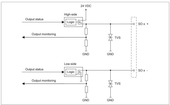
Figure 6: Type A output circuit diagram
