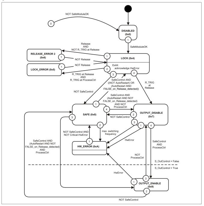
Figure 7: Restart interlock - State diagram
