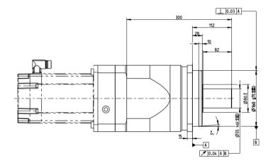
Spline shaft according to DIN 5480 - W 55 x 2 x 30 x 26 x 6 m  $\,$
