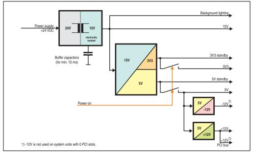
Figure 17: Block diagram - supply voltage
