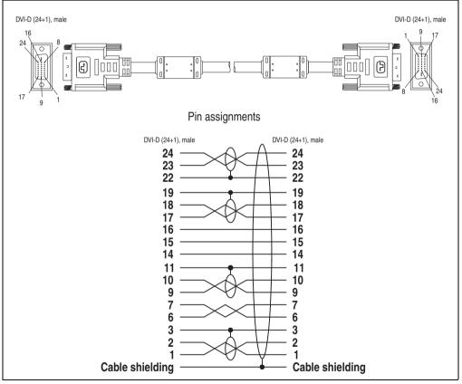
Figure 337: Pin assignments - DVI cable
