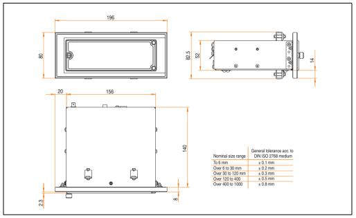
Figure 317: Dimensions - USB Media Drive with front cover
