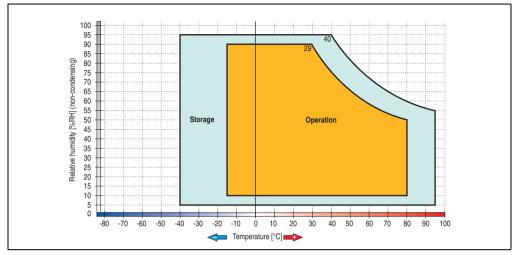
Figure 141: Temperature humidity diagram - SATA RAID hard disk 5ACPCI.RAIC-04
