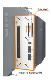
Figure 386: Example - Side cover removal on the system unit 5PC720.1505-02
