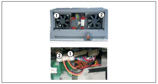
Figure 382: Fan cable connection on the main board
