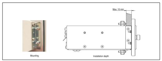
Figure 331: Front cover mounting and installation depth
