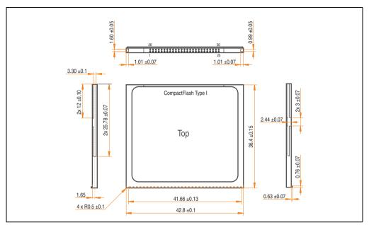
Figure 308: Dimensions - CompactFlash card Type I
