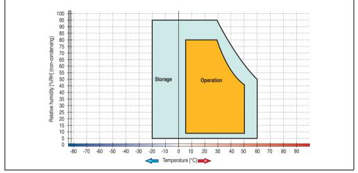
Figure 116: Temperature humidity diagram - Slide-in DVD-ROM/CD-RW 5AC600.DVDS-00
