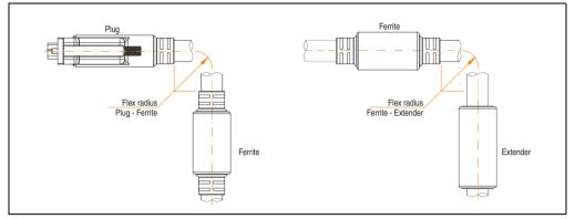
Figure 353: Flex radius specification
