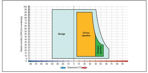
Figure 131: Temperature humidity diagram - RAID hard disk 5ACPCI.RAIS-00
