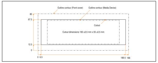
Figure 326: Installation cutout - USB Media Drive with front cover
