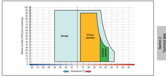
Figure 137: Temperature humidity diagram - SATA RAID hard disk 5ACPCI.RAIC-02
