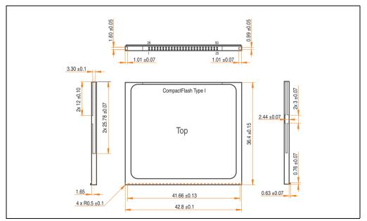
Figure 299: Dimensions - CompactFlash card Type I
