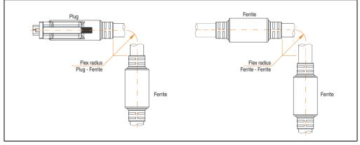
Figure 336: Flex radius specification
