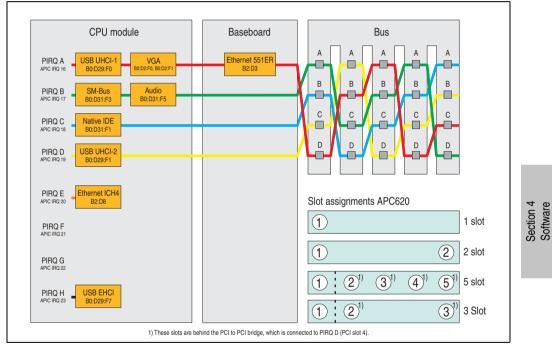
Figure 274: PCI routing with activated APIC CPU boards 815E (ETX), 855GME (ETX)
