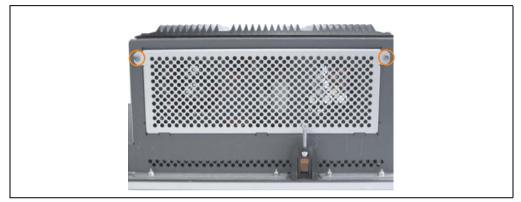
Figure 378: Removing the fan kit cover
