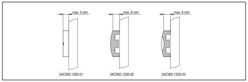
Figure 297: USB port cap (attached) - Height
