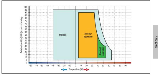
Figure 107: Temperature humidity diagram - Add-on hard disk 5AC600.HDDI-04
