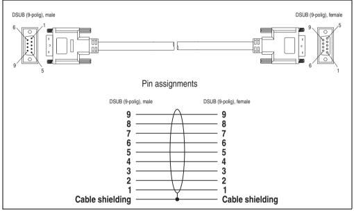
Figure 358: Pin assignments - RS232 cable
