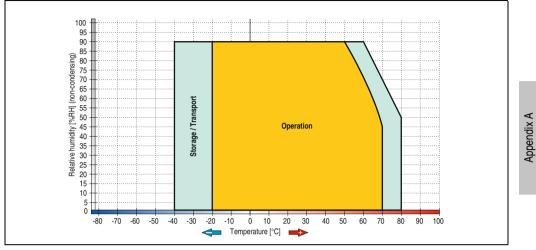
Figure 398: Temperature humidity diagram - AMT touch screen
