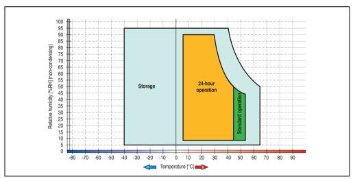
Figure 123: Temperature humidity diagram - Slide-in hard disk 5AC600.HDDS-00
