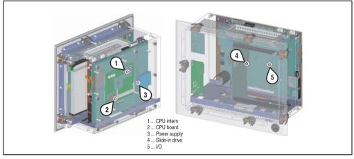
Figure 392: Temperature sensor locations
