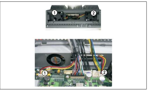
Figure 377: Fan cable connection on the main board
