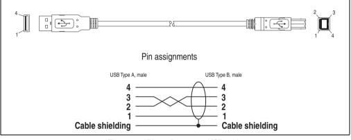
Figure 360: Pin assignments - USB cable
