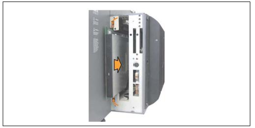
Figure 388: Installing the slide-in drive
