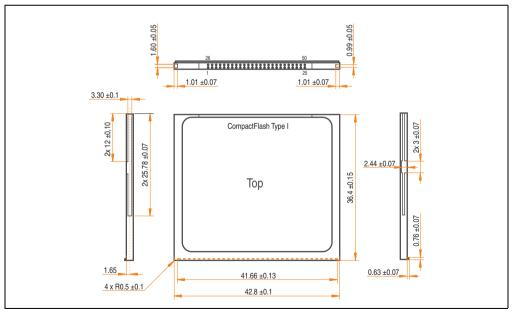
Figure 303: Dimensions - CompactFlash card Type I
