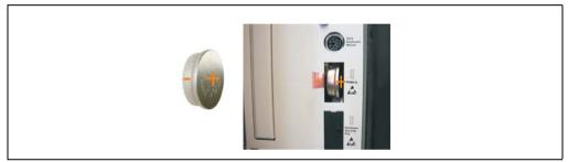
Figure 371: Battery polarity
