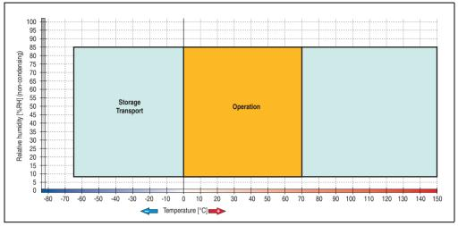
Figure 298: Temperature humidity diagram - CompactFlash cards 5CFCRD.xxxx-06
