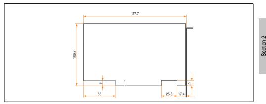
Figure 32: Dimensions - Standard half-size PCI cards
