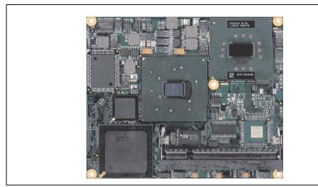
Figure 87: CPU boards 855GME (XTX)
