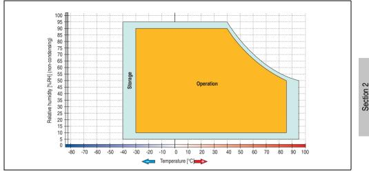
Figure 111: Temperature humidity diagram - Add-on hard disk 5AC600.HDDI-06
