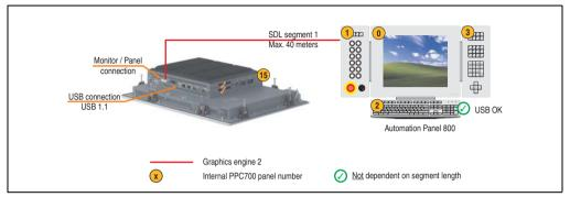
Figure 159: Configuration - An Automation Panel 800 via SDL (onboard)
