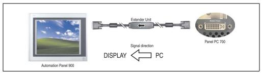
Figure 346: Example of signal direction for the SDL cable with extender - PPC700
