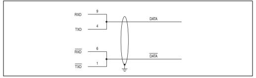
Figure 148: Add-on RS232/422/485 interface - operated in RS485 mode
