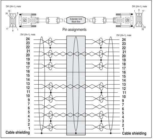
Figure 347: Pin assignments - SDL cable with extender 5CASDL.0x00-10
