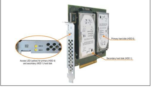
Figure 134: PCI SATA RAID controller - 5ACPCI.RAIC-01
