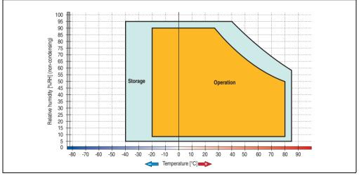
Figure 125: Temperature humidity diagram - Slide-in hard disk 5AC600.HDDS-01
