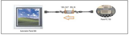
Figure 355: Example of signal direction for the SDL flex cable with extender - PPC700
