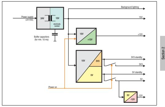
Figure 23: Block diagram - supply voltage
