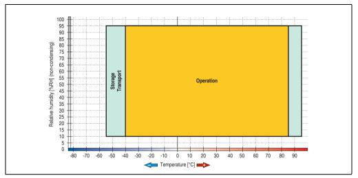
Figure 97: Temperature humidity diagram - Replacement SSD 128 GB - 5MMSSD.0128-00  $\ge$  E0
