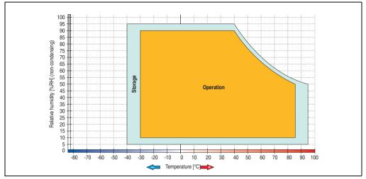
Figure 109: Temperature humidity diagram - Add-on hard disk 5AC600.HDDI-05
