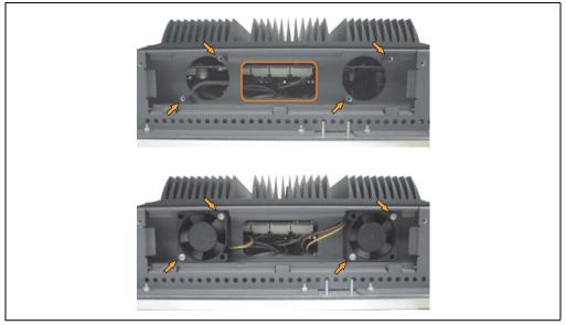
Figure 375: Fan Installation
