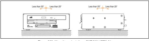
Figure 328: Mounting orientation - 5MD900.USB2-01
