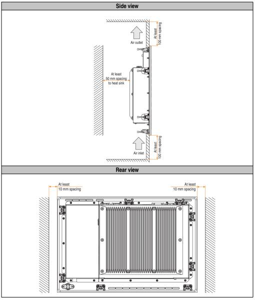
Figure 154: Spaces for air circulation
