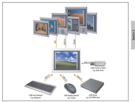
Figure 164: Remote connection of USB peripheral devices to the APC900 via DVI
