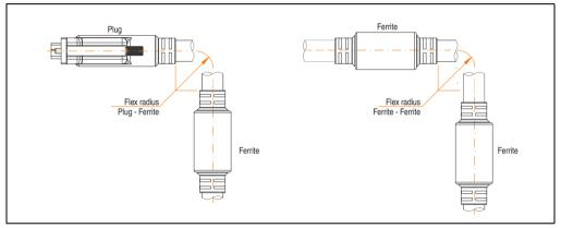
Figure 349: Flex radius specification
