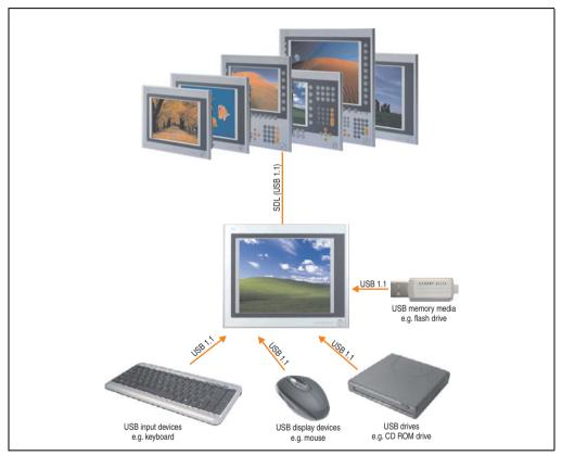
Figure 165: Remote connection of USB peripheral devices to the APC800/900 via SDL
