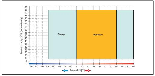
Figure 306: Temperature humidity diagram - CompactFlash cards 5CFCRD.xxxx-03
