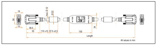
Figure 354: Dimensions - SDL flex cable with extender 5CASDL.0x00-13
