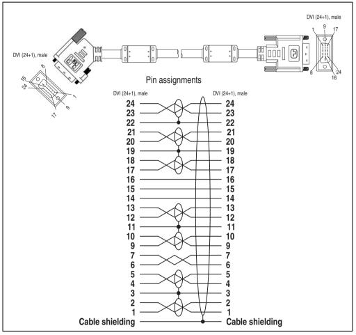
Figure 343: Pin assignments - SDL cable with 45° plug 5CASDL.0xxx-01
