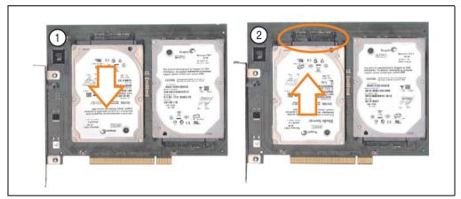
Figure 391: Hard disk exchange
