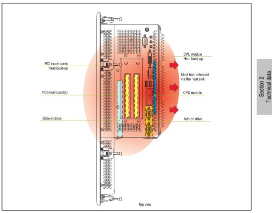
Figure 4: Example of worst-case conditions for temperature measurement
