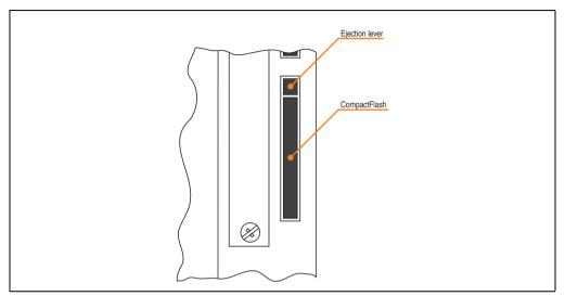
Figure 372: CompactFlash + ejection lever (representation picture)
