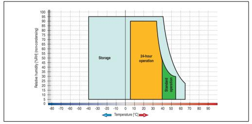
Figure 135: Temperature humidity diagram - SATA RAID hard disk 5ACPCI.RAIC-01
