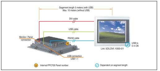
Figure 157: Configuration - One Automation Panel via DVI (onboard)
