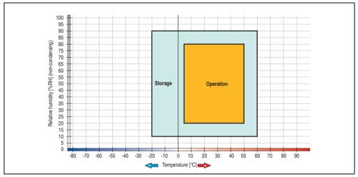
Figure 121: Temperature humidity diagram - Slide-in USB diskette drive 5AC600.FDDS-00
