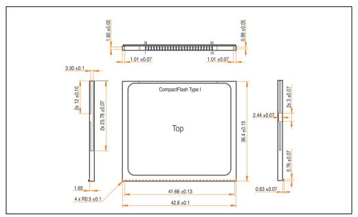
Figure 307: Dimensions - CompactFlash card Type I
