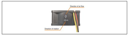
Figure 374: Marking for direction of airflow / fan rotation
