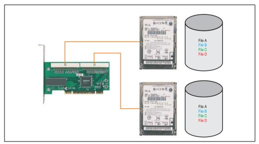
Figure 128: RAID 1 system schematic
