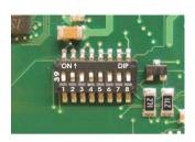
Figure 213: DIP switch on system unit
