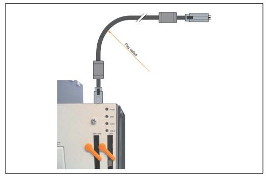
Figure 155: Flex radius - Cable connection
