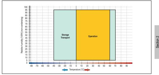
Figure 145: Temperature humidity diagram - SATA RAID hard disk - 5MMHDD.0250-00
