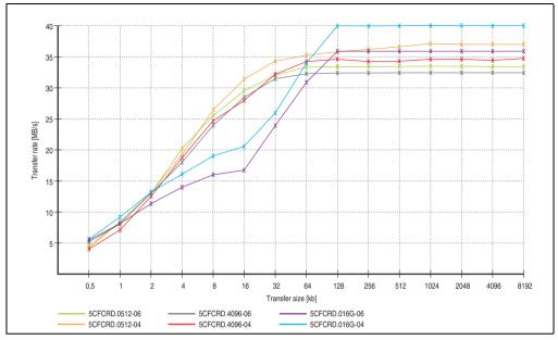
Figure 300: ATTO Benchmark v2.34 comparison when reading - 5CFCRD.xxxx-04 with 5CFCRD.xxxx-06
