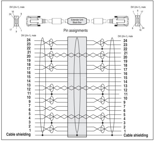
Figure 356: Pin assignments - SDL flex cable with extender 5CASDL.0x00-13
