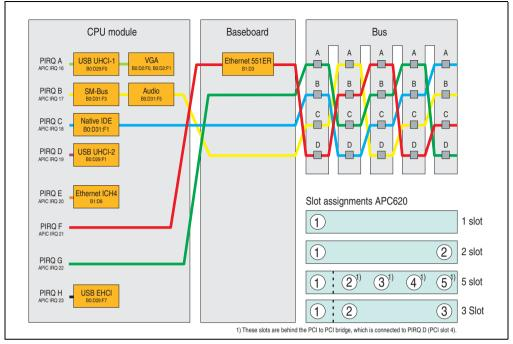
Figure 275: PCI routing with activated APIC CPU boards 855GME (XTX)
