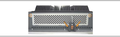
Figure 373: Removing the fan kit cover
