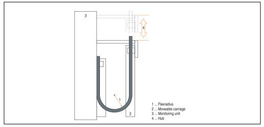
Figure 292: Test structure - Cable drag chain
