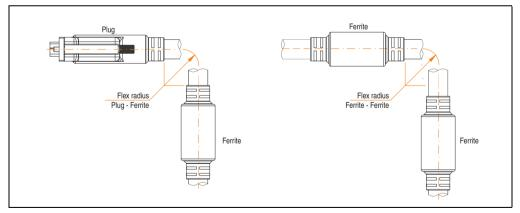
Figure 339: Flex radius specification
