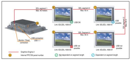
Figure 161: Configuration - Four Automation Panel 900 units via SDL (onboard)
