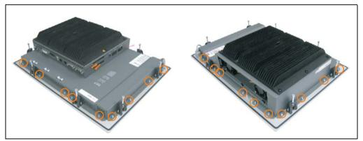
Figure 376: Removing the cover
