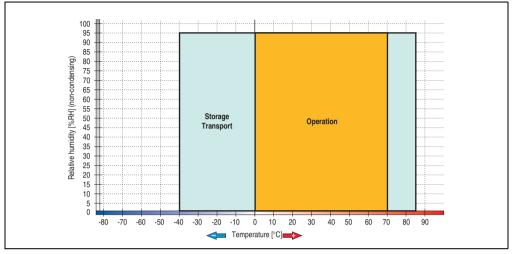
Figure 92: Temperature humidity diagram - Add-on SSD 128 GB - 5AC600.SSDI-00  $\leq$  D0
