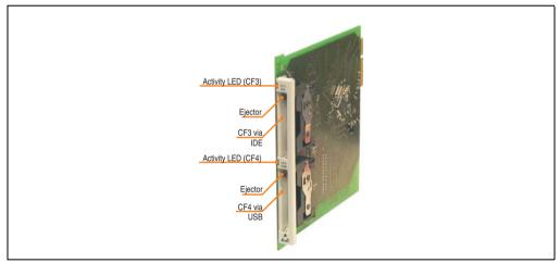
Figure 119: Slide-in CF 2-slot - 5AC600.CFSS-00
