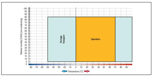
Figure 333: Temperature humidity diagram - USB flash drive - 5MMUSB.2048-01
