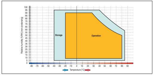
Figure 101: Temperature humidity diagram - Add-on hard disk 5AC600.HDDI-01
