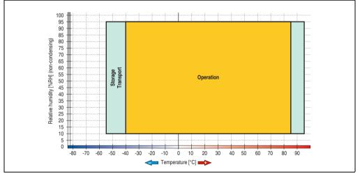
Figure 93: Temperature humidity diagram - Add-on SSD 128 GB - 5AC600.SSDI-00  $\geq$  E0
