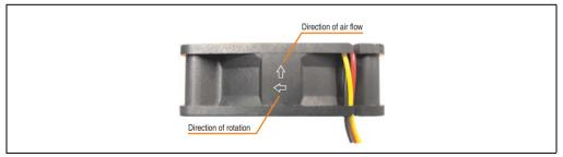
Figure 379: Marking for direction of airflow / fan rotation
