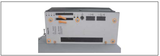
Figure 381: Removing the side cover
