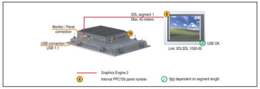
Figure 158: Configuration - An Automation Panel 900 via SDL (onboard)
