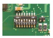
Figure 242: DIP switch on system unit
