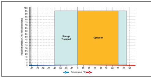
Figure 96: Temperature humidity diagram - Replacement SSD 128 GB - 5MMSSD.0128-00  $\leq$  D0
