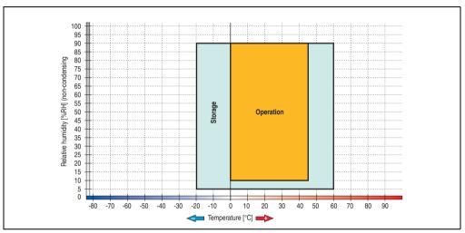
Figure 332: Temperature humidity diagram - USB flash drive - 5MMUSB.2048-00
