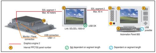
Figure 160: Configuration - One AP900 and an AP800 via SDL (onboard)
