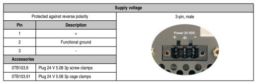
Figure 29: Supply voltage connection
