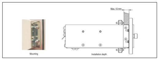
Figure 322: Front cover mounting and installation depth
