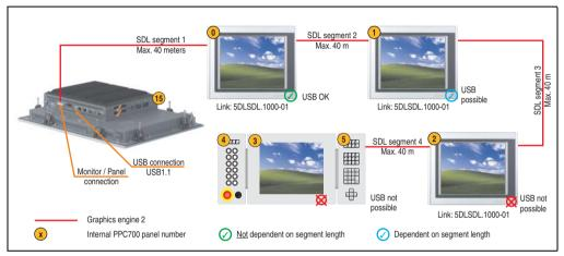
Figure 162: Three Automation Panel 900 devices and an Automation Panel 800 via SDL (onboard)
