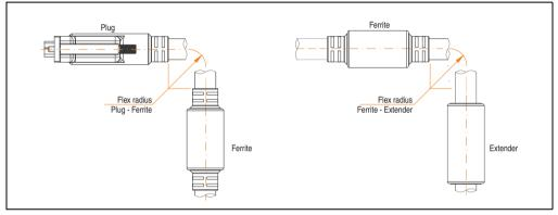
Figure 345: Flex radius specification
