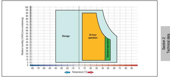
Figure 99: Temperature humidity diagram - Add-on hard disk 5AC600.HDDI-00
