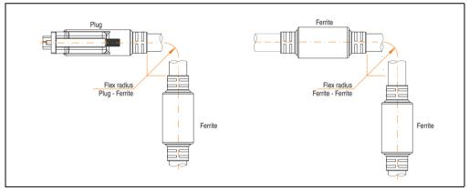
Figure 342: Flex radius specification
