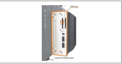
Figure 383: Example - Side cover removal on the system unit 5PC720.1505-02
