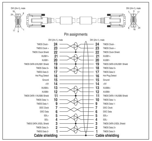
Figure 351: Pin assignments - SDL cable 5CASDL.0xxx-03
