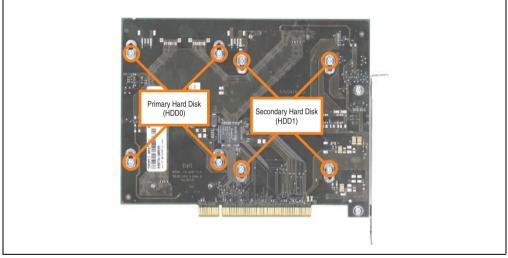
Figure 390: Screw assignment on the back side of the SATA RAID controller
