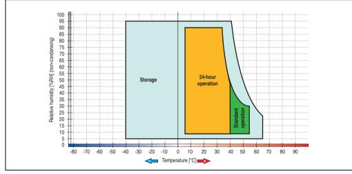
Figure 133: Temperature humidity diagram - RAID hard disk 5ACPCI.RAIS-01
