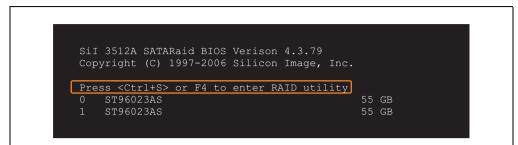
Figure 166: Open the RAID Configuration Utility
