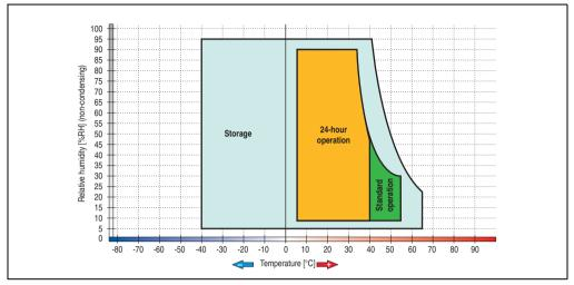
Figure 105: Temperature humidity diagram - Add-on hard disk 5AC600.HDDI-03
