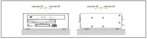
Figure 319: Mounting orientation - 5MD900.USB2-00
