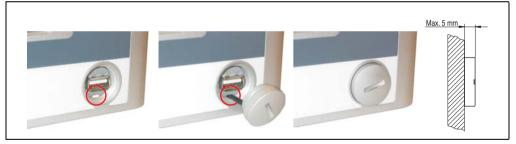
Figure 296: Front side USB port cap - installation
