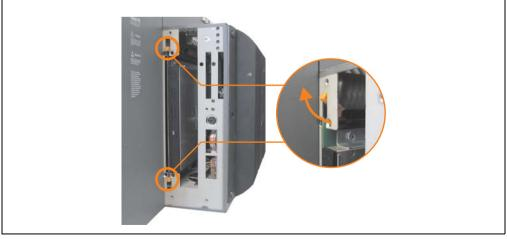
Figure 387: Release the slide-in slot releasing mechanisms
