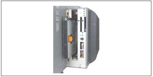
Figure 385: Installing the slide-in drive
