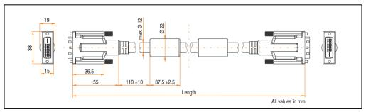
Figure 350: Dimensions - SDL cable 5CASDL.0xxx-03
