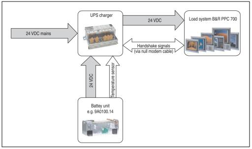
Figure 294: Block diagram of the UPS
