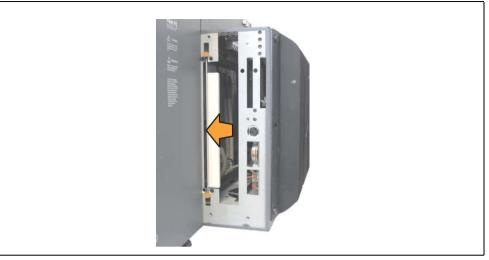
Figure 384: Removing the slide-in dummy module
