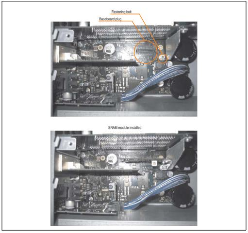
Figure 364: SRAM module installation
