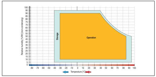
Figure 127: Temperature humidity diagram - Slide-in hard disk 5AC600.HDDS-02
