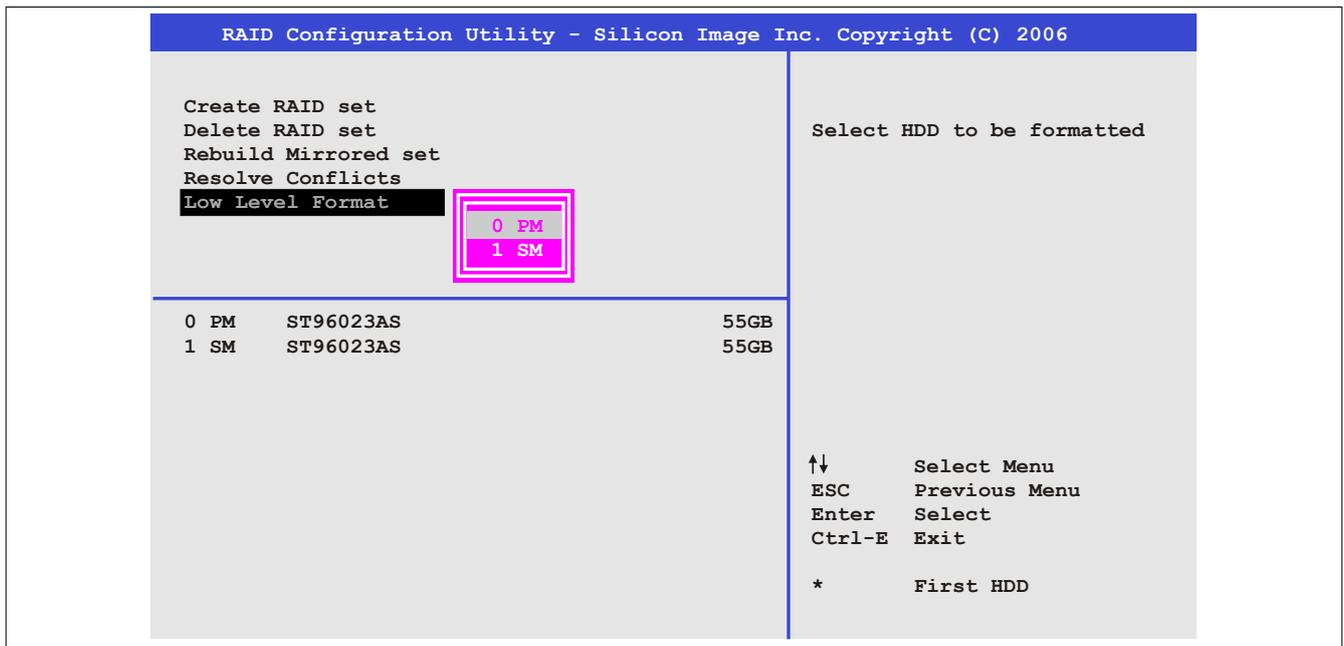
Abbildung 79: RAID Configuration Utility - Low Level Format
