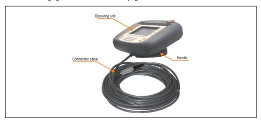
Figure 42: Attachment cable and handle
