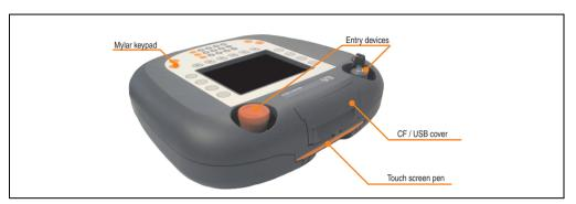
Figure 7: Mobile Panel operating unit
