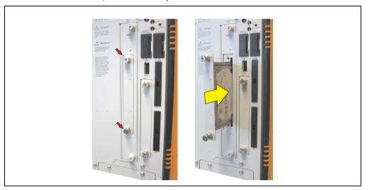
Figure 197: Mounting the slide-in compact drive
