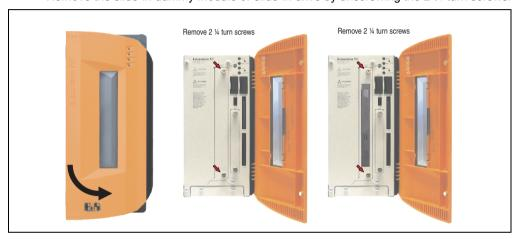
Figure 193: Loosening the 1/4 turn screws
