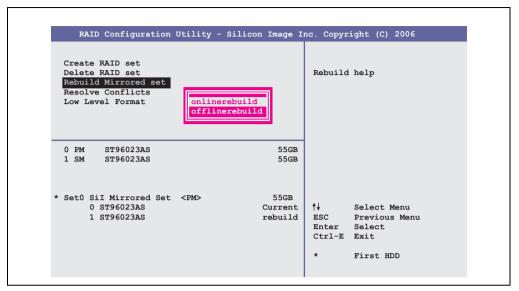
Figure 97: RAID Configuration Utility - Rebuild Mirrored set
