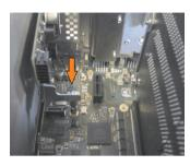
Figure 216: Install UPS module
