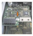
Figure 221: Install UPS module
