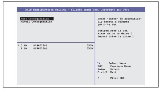
Figure 94: RAID Configuration Utility - Create RAID set - striped
