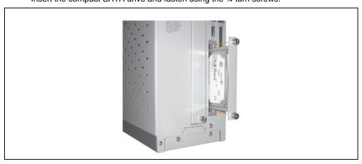
Figure 192: Inserting the compact SATA drive
