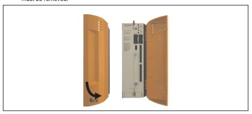
Figure 236: Mounting the side cover - APC810 1 card slot
