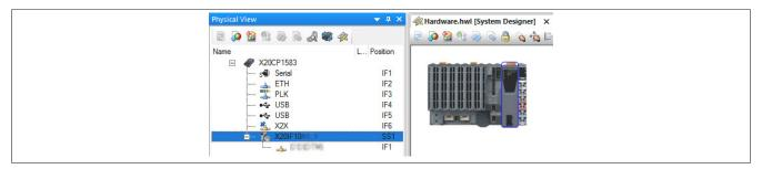
• Additional module settings can be made under "Device configuration". This configuration environment is opened by right-clicking on the IF interface and selecting "Device configuration".
