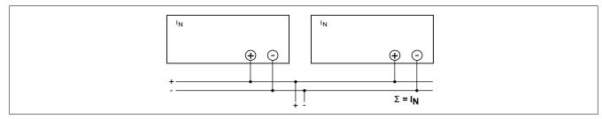
Redundant connections are designed for supplying systems with particularly high requirements on operational safety. If a fault occurs in the primary circuit of the first power supply unit, the second device automatically takes over the complete power supply without interruption, and vice versa.
