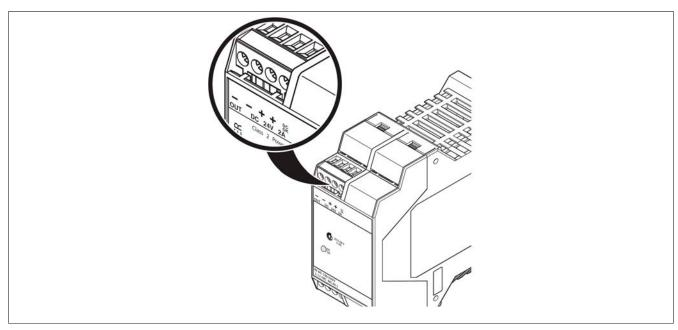
The connection is made via the "+" and "-" screw connectors on the DC output. The configured output voltage upon delivery is 24 VDC. The output voltage can be configured using the potentiometer.
