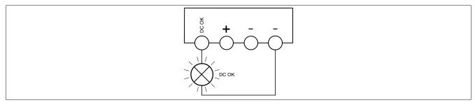
The 24 VDC signal is between the connection terminals "DC OK" and "-" and can carry up to 20 mA. This signal output changes from "active high" to "low" to indicate the voltage has fallen below the 21.5 VDC output voltage.
