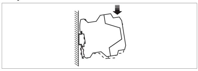
Position the module with the DIN rail guide on the **upper edge** of the DIN rail, and snap it in with a **downward** motion.
