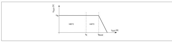
The device provides the rated output current  $I_N$  up to an ambient temperature of 60°C. At an ambient temperature of up to 40°C, the unit supplies a continuous output current of  $I_N$ . The operating point follows the U/I curve when a heavy load is applied.
