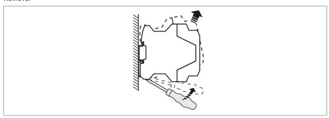
Pull the snap lever open with the aid of a screwdriver and slide the module out at the **lower edge** of the DIN rail.
