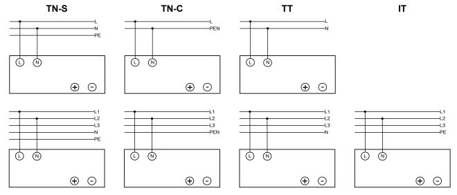
The 100 to 240 VAC connection is made using the L and N screw connections.
