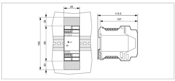
Installation depth 107 mm + DIN rail
