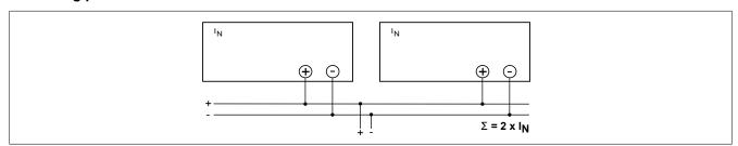
The output current can be increased to  $n \times I_N$  where n is the number of devices connected in parallel.
