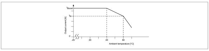
The device provides the rated output current  $I_N$  up to an ambient temperature of 60°C. At an ambient temperature of up to 40°C, the unit supplies a continuous output current of  $I_N$ .
