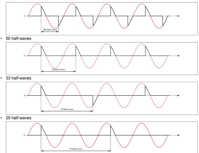
With multichannel operation, the second channels should be operated with delayed half-waves in order to ensure that the load is placed evenly on the module.
