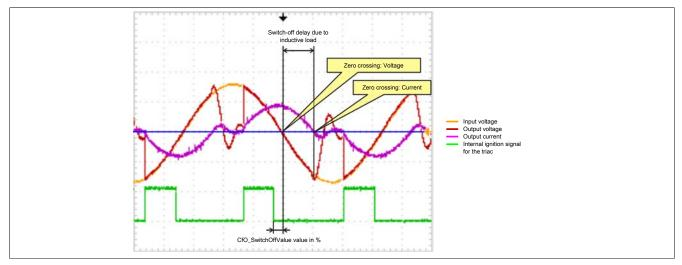
With inductive loads, a suitable varistor must be provided between the output DO x and the phase L (e.g. a varistor with 275  $V_{RMS}$  at 240 VAC).
