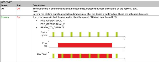
Table: LED "S/E" - Error message (interface in POWERLINK mode)
