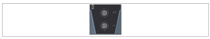
The node number for the POWERLINK station is set using the two number switches. The node number can also be directly configured using Automation Studio.
