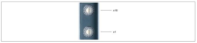
The X2X Link address of the module is set using the node number switches (0x01 to 0xFD).
