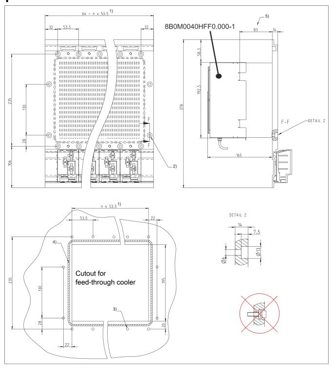
Figure 1: Dimension diagram and installation dimensions
