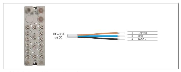
① X67CA0D40.xxxx: M8 sensor cable, straight X67CA0D50.xxxx: M8 sensor cable, angled
