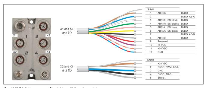
X67CA0I41.xxxx: Straight multi-function cable X67CA0I51.xxxx: Angled multi-function cable M12 straight sensor cable X67CA0A51.xxxx: M12 angled sensor cable
