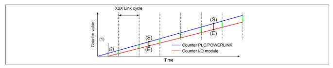
At startup, the internal counters for the PLC/POWERLINK (1) and the I/O module (2) start at different times and increase the values at  $\mu$ s intervals.
