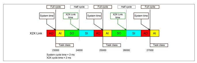
The reference time on the X2X Link network is always formed at the half cycle of the X2X Link cycle. This results in a difference between the system time and the X2X Link reference time when the reference time is read out.
