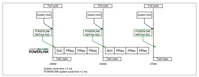
The reference time at POWERLINK is always formed at the SoC (Start of Cycle) of the POWERLINK network. The SoC starts 20 µs after the system tick. This results in the following difference between the system time and the POWERLINK reference time:
