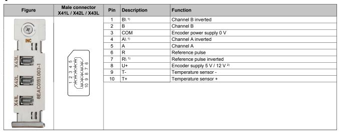
Table 3: Incremental encoder interface 8EAC0151.003-1 - Pinout
