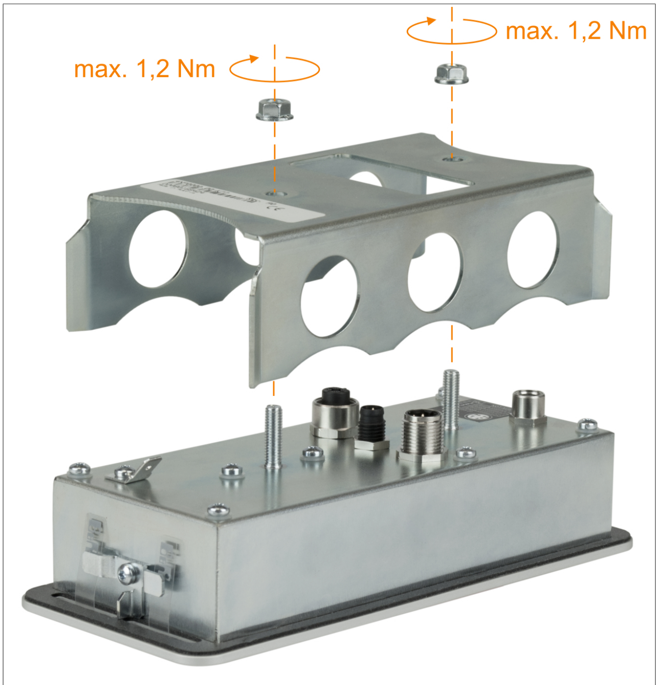
Figure 5: 4XP0000.00-K76 - Installation guidelines
