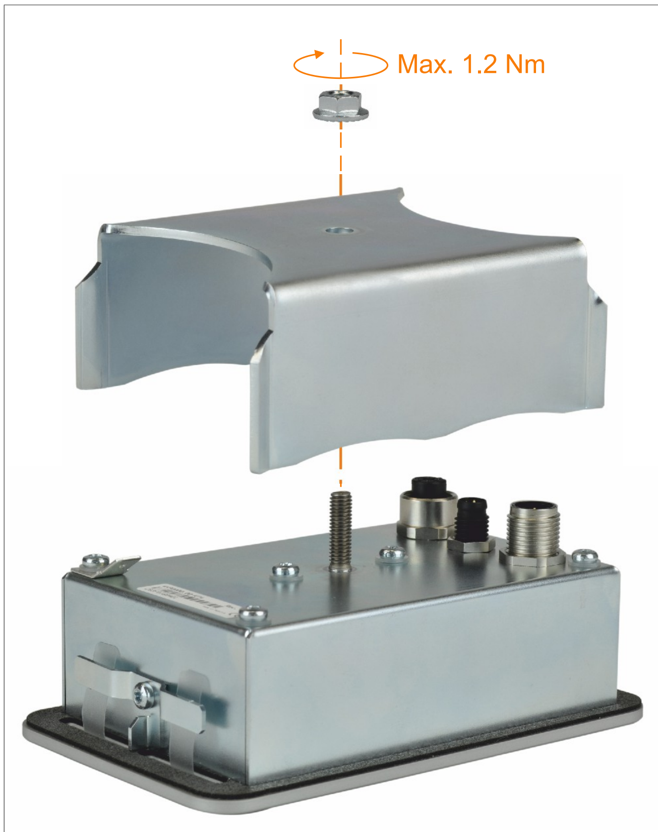
Figure 6: 4XP0000.00-K64 - Installation guidelines
