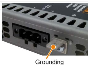
The ground connection must be used, for example, to fasten a copper strip to a central grounding point in the control cabinet or system where the device is installed. The largest possible conductor cross section should be used (at least 2.5 mm<sup>2</sup>).
