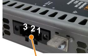
Table 18: +24 VDC voltage supply connection
