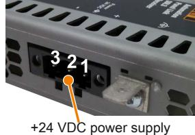
Table 21: +24 VDC voltage supply connection
