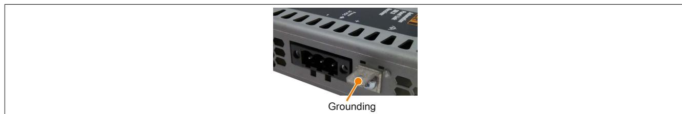
The ground connection must be used, for example, to fasten a copper strip to a central grounding point in the control cabinet or system where the device is installed. The largest possible conductor cross section should be used (at least 2.5 mm<sup>2</sup>).
