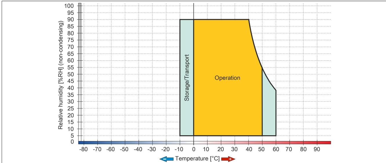
Figure 27: 5AP99D.185B-0x - Temperature/Humidity diagram
