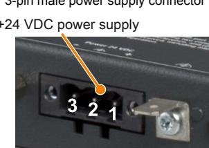
Table 33: +24 VDC voltage supply connection
