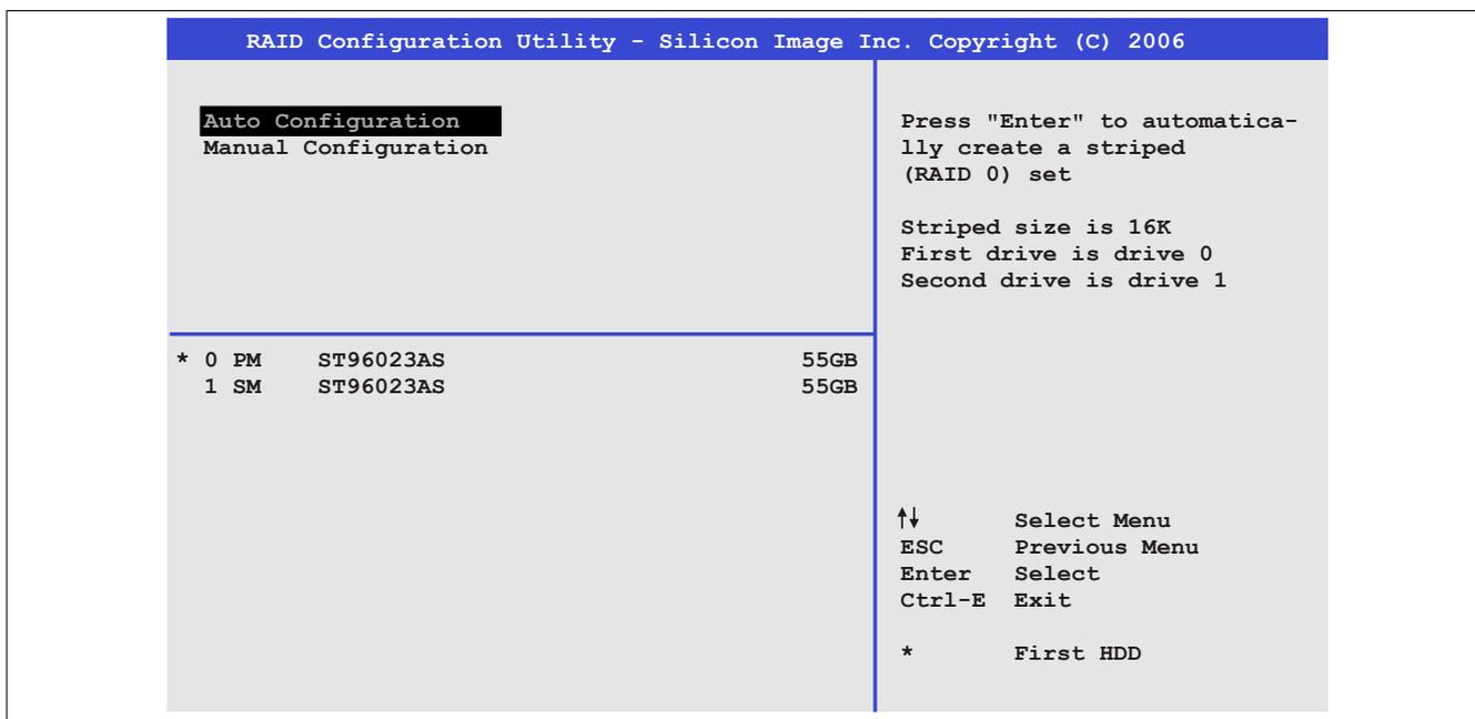
Abbildung 73: RAID Configuration Utility - Create RAID set - Striped
