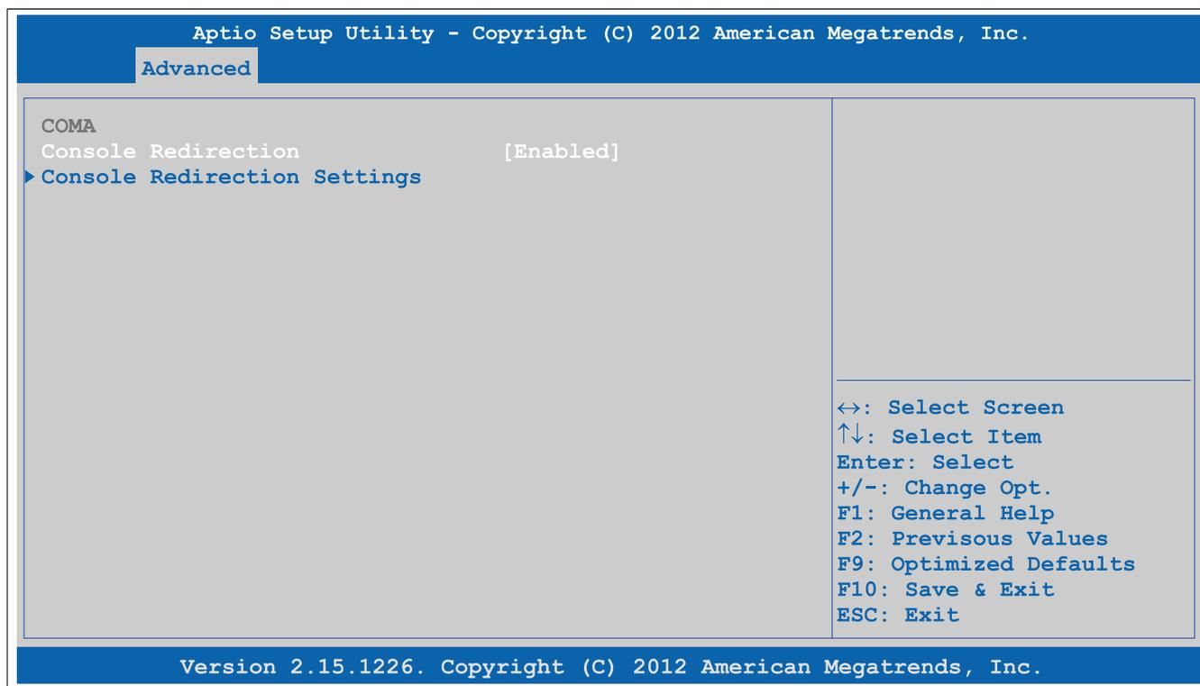
Abbildung 138: Advanced - Serial Port Console Redirection
