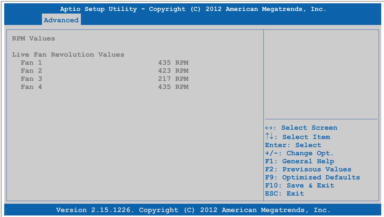
Abbildung 111: Advanced - OEM Features - Fan Unit Features - RPM Values
