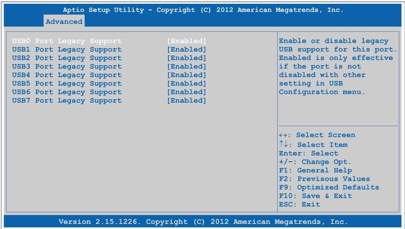
Abbildung 137: Advanced - USB Configuration - Per Port Legacy USB Support Control
