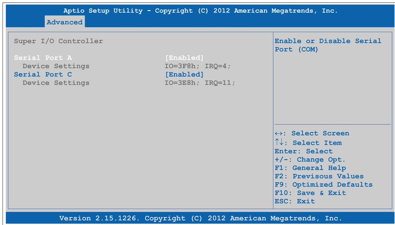
Abbildung 92: Advanced - OEM Features - Super I/O Configuration
