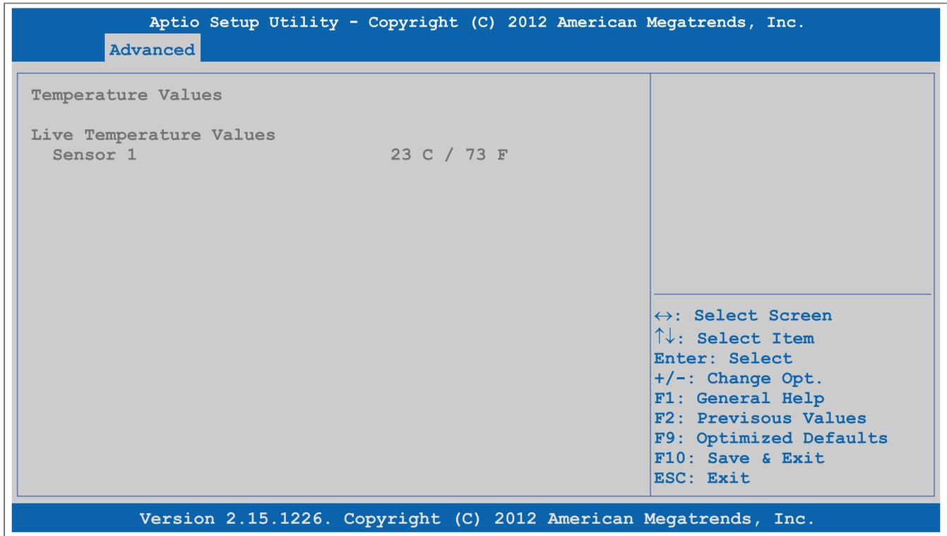
Abbildung 113: Advanced - OEM Features - Slide-in 1 Features - Temperature Values
