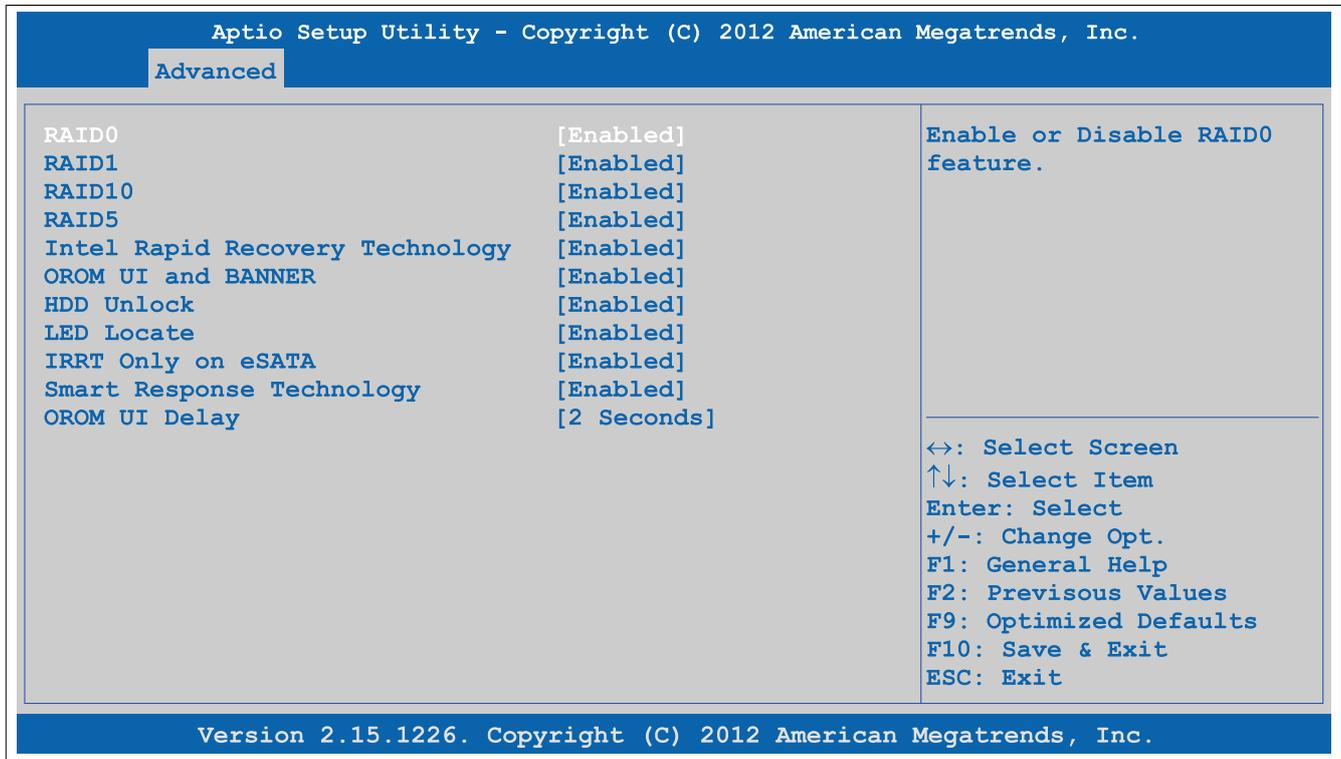
Abbildung 131: Advanced - SATA Configuration - Software Feature Mask Configuration
