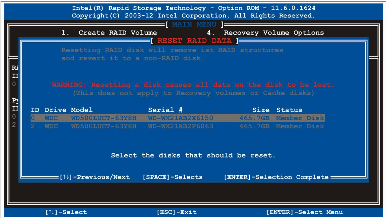
Abbildung 83: Configuration Utility - Reset Disks to Non-RAID
