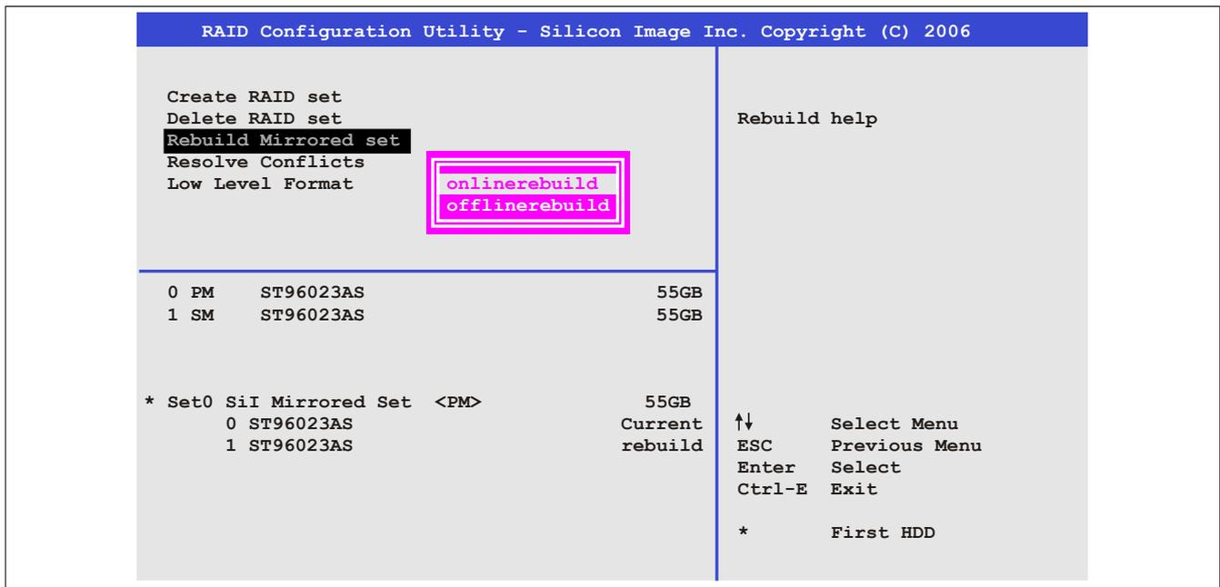
Abbildung 76: RAID Configuration Utility - Rebuild Mirrored set
