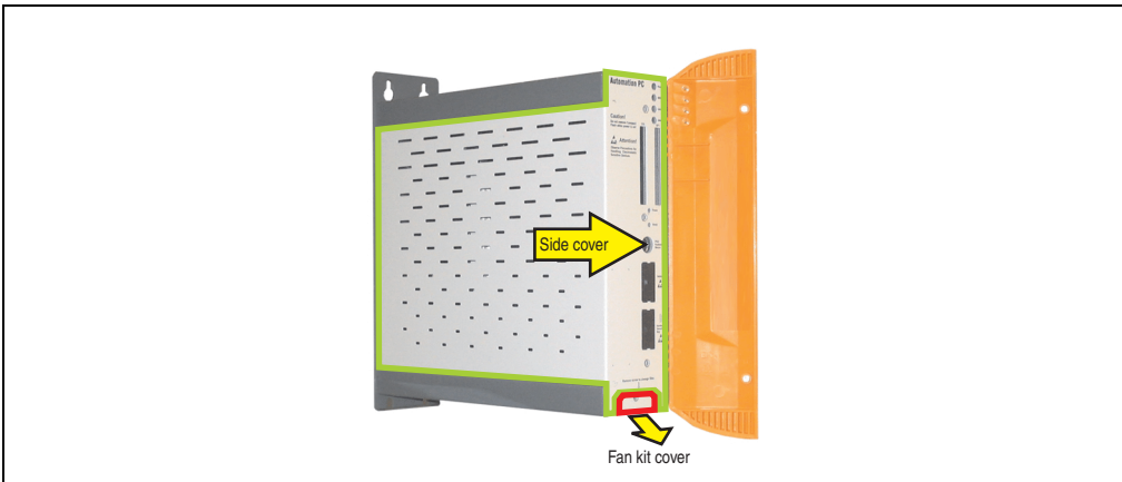
Figure 388: APC620 1PCI slot - Remove side cover and fan kit cover
