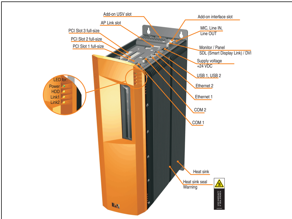
Figure 13: Interface overview - APC620, 3 PCI slot variant (top)
