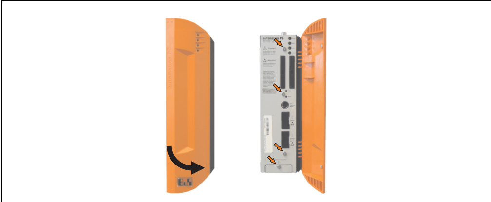
Figure 387: APC620 1PCI slot - Remove screws to install/ remove filter kit
