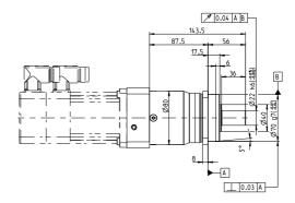
Spline shaft according to DIN 5480 - W 22 x 0.8 x 30 x 26 x 7 m
