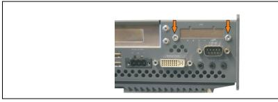
Figure 425: Remove UPS module cover
