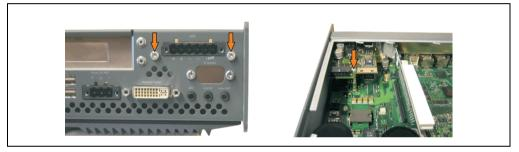
Figure 408: Install UPS module
