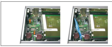
Figure 435: Plug in connection cable
