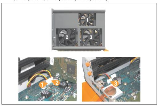
Figure 398: APC620 5PCI slot - Fan cable connection to the main board
