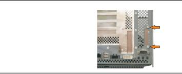
Figure 437: Remove UPS module cover
