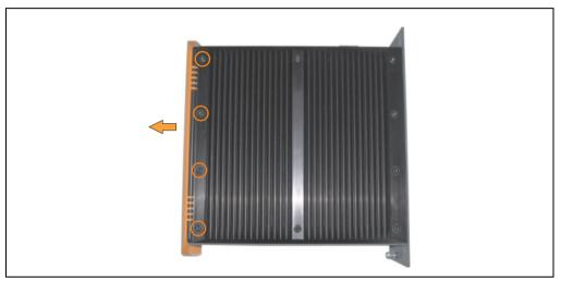
Figure 450: Removing the APC620 front cover
