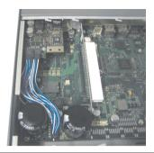
Figure 428: Plug in connection cable
