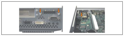
Figure 427: Install UPS module
