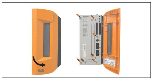
Figure 381: APC620 2PCI slots - Remove screws to install/ remove filter kit
