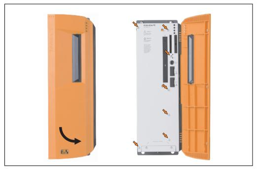
Figure 446: Mounting the side cover - APC620, 3 PCI slot
