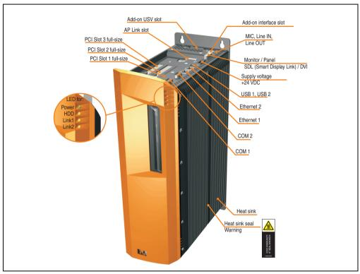
Figure 13: Interface overview - APC620, 3 PCI slot variant (top)
