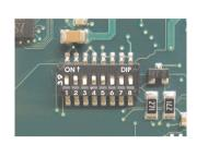
Figure 247: DIP switch on system unit
