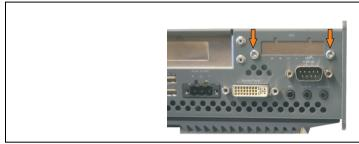
Figure 420: Remove UPS module cover
