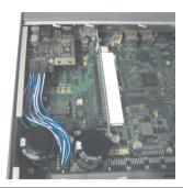
Figure 423: Plug in connection cable
