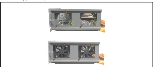
Figure 379: APC620 2PCI slots - Fan installation
