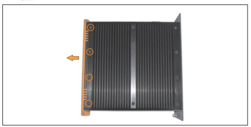
Figure 445: Removing the APC620 front cover
