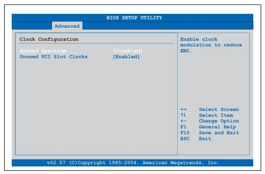
Figure 226: 855GME (XTX) Advanced Clock Configuration
