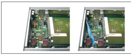
Figure 430: Plug in connection cable
