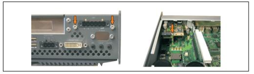
Figure 403: Install UPS module
