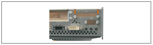
Figure 401: Remove UPS module cover
