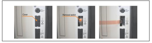
Figure 238: Battery removal
