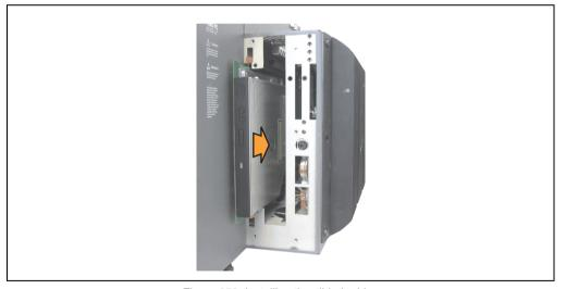
Figure 253: Installing the slide-in drive
