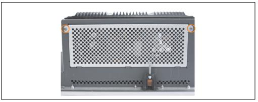
Figure 246: Removing the fan kit cover
