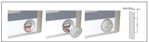
Figure 183: Front side USB port cap - installation
