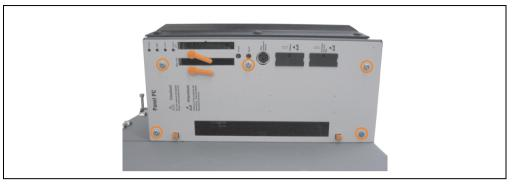
Figure 249: Removing the side cover
