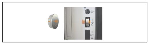
Figure 240: Battery polarity
