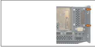
Figure 247: Remove UPS module cover
