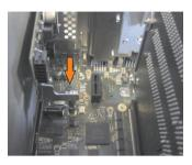
Figure 256: Install UPS module
