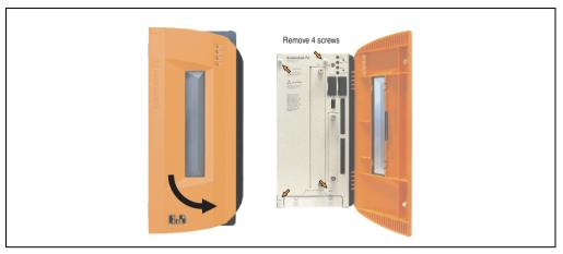
Figure 277: Mounting the side cover - APC810 2 card slot
