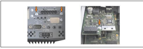
Figure 244: Install UPS module
