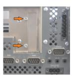
Figure 279: Remove AP Link module cover
