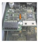
Figure 261: Install UPS module
