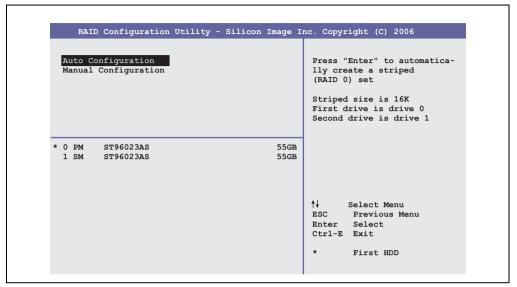
Figure 106: RAID Configuration Utility - Create RAID set - Striped
