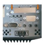
Figure 259: Remove UPS module cover
