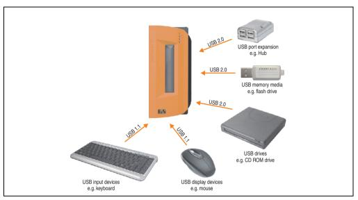
Figure 100: Local connection of USB peripheral devices on the APC810
