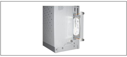
Figure 232: Inserting the compact SATA drive
