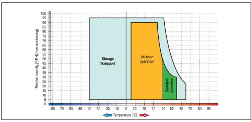
Figure 101: Temperature humidity diagram - SATA RAID hard disk 5ACPCI.RAIC-01
