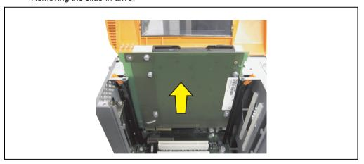
Figure 398: Removing the slide-in drive
