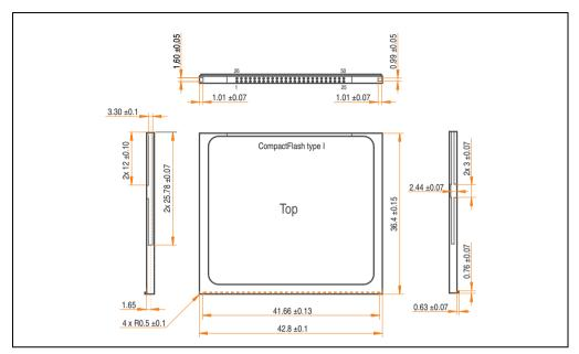
Figure 295: Dimensions - CompactFlash card Type I
