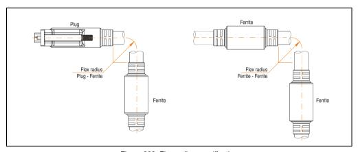
Figure 323: Flex radius specification
