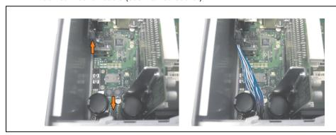
Figure 418: Plug in connection cable
