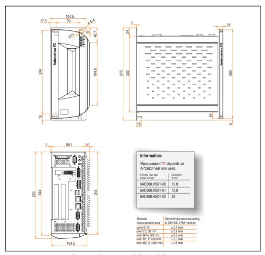
Figure 12: Dimensions - APC620, 2 PCI slot variant
