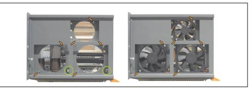
Figure 392: APC620 5PCI slot - Fan installation
