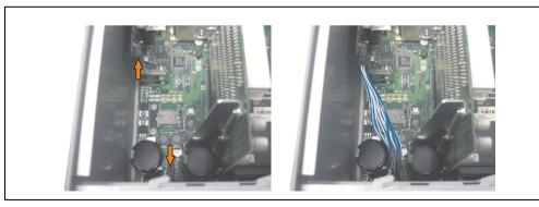
Figure 437: Plug in connection cable
