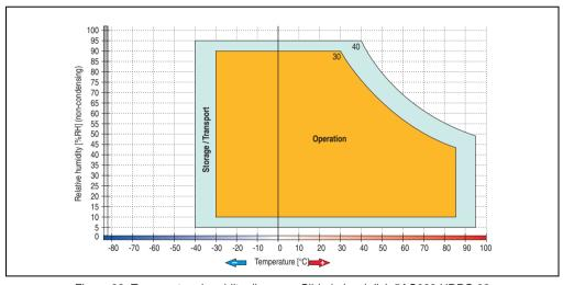
Figure 93: Temperature humidity diagram - Slide-in hard disk 5AC600.HDDS-02
