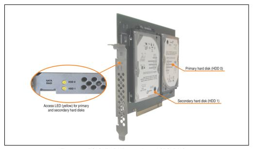
Figure 100: PCI SATA RAID controller - 5ACPCI.RAIC-01
