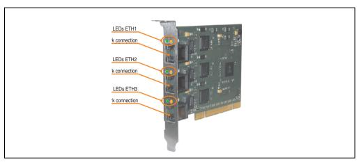
Figure 362: PCI Ethernet card 10/100 - 5ACPCI.ETH3-01
