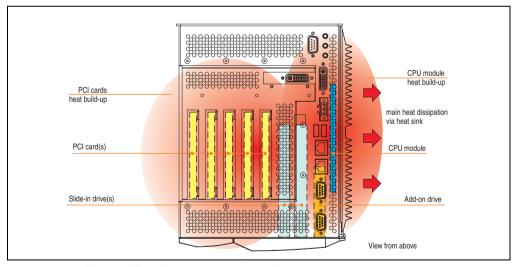
Figure 24: Example of worst-case conditions for temperature measurement
