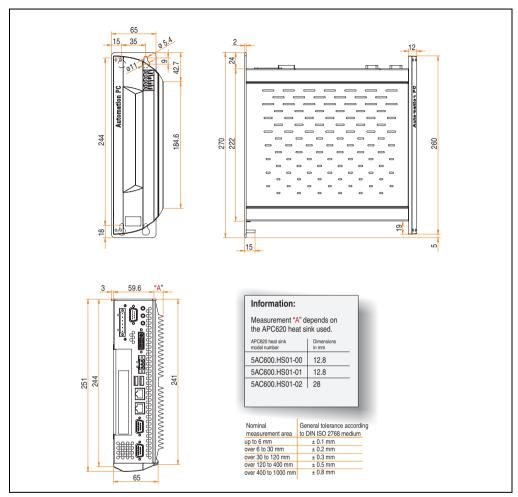
Figure 9: Dimensions - APC620, 1 PCI slot variant
