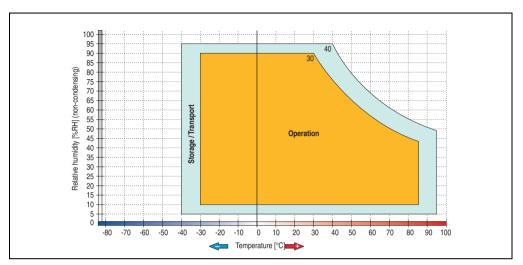
Figure 75: Temperature humidity diagram - Add-on hard disk 5AC600.HDDI-05
