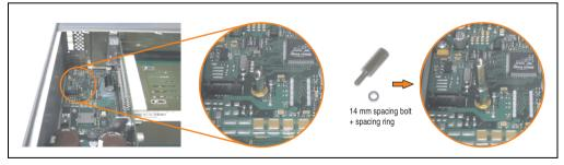
Figure 408: Screw in spacing bolt and spacing ring
