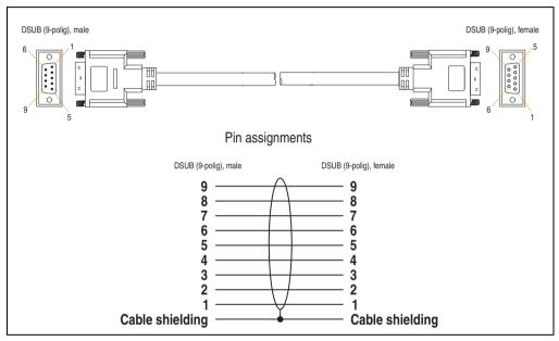
Figure 346: Pin assignments - RS232 cable
