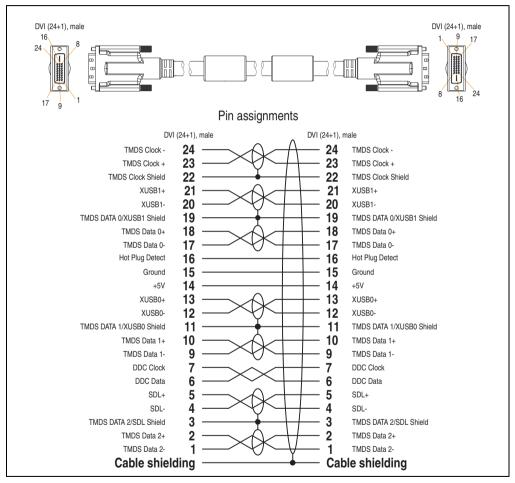
Figure 338: Pin assignments - SDL cable 5CASDL.0xxx-03
