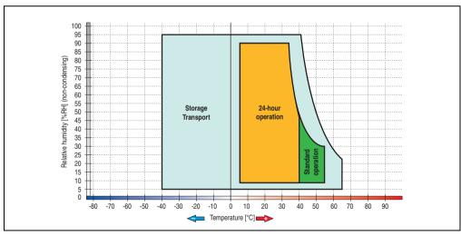
Figure 97: Temperature humidity diagram - RAID hard disk 5ACPCI.RAIS-00
