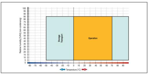
Figure 319: Temperature humidity diagram - USB flash drive - 5MMUSB.2048-01
