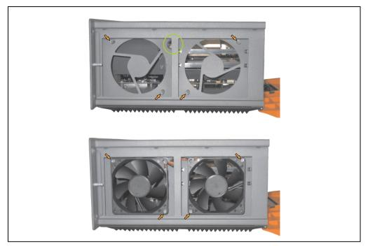
Figure 385: APC620 3PCI slot - Fan installation
