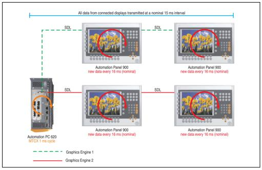
Figure 453: Sample configuration for SDL timing
