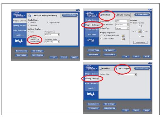
Figure 268: Dual display clone settings - primary and secondary device
