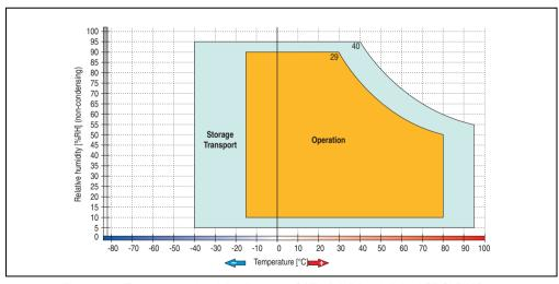
Figure 106: Temperature humidity diagram - SATA RAID hard disk 5ACPCI.RAIC-03
