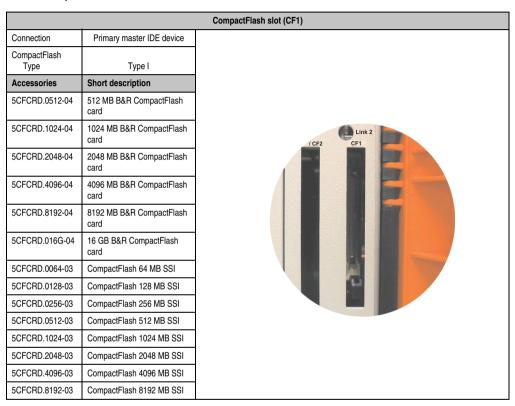
Table 64: Technical data - CompactFlash slot (CF1)
