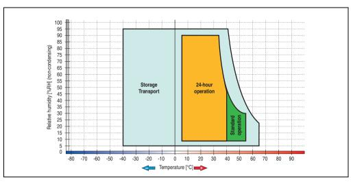
Figure 69: Temperature humidity diagram - Add-on hard disk 5AC600.HDDI-02
