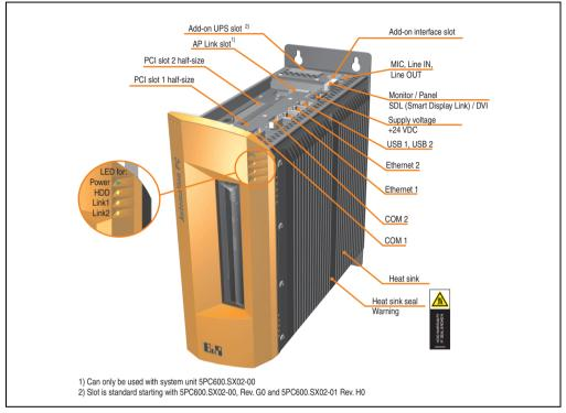
Figure 10: Interface overview - APC620, 2 PCI slot variant (top)
