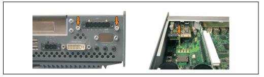
Figure 403: Install UPS module
