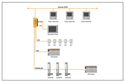
Figure 1: APC620 embedded for central control and visualization
