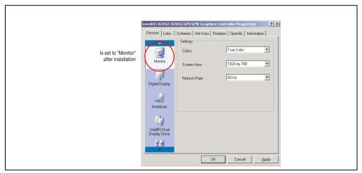
Figure 269: Settings after installing the graphics driver
