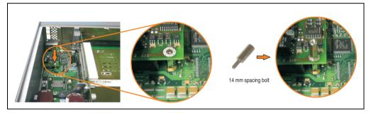
Figure 427: Screw in spacing bolt
