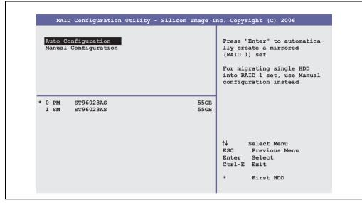
Figure 150: RAID Configuration Utility - Create RAID set - Mirrored
