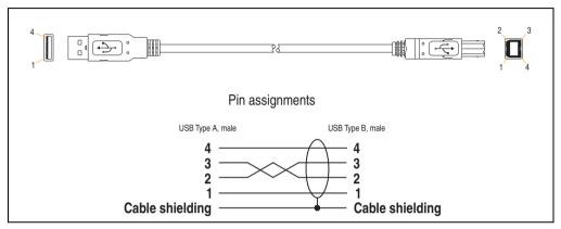
Figure 348: Pin assignments - USB cable
