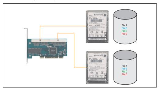
Figure 94: RAID 1 system schematic
