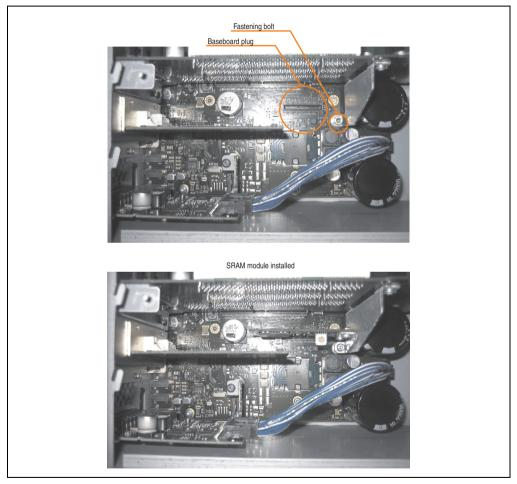
Figure 366: SRAM module installation
