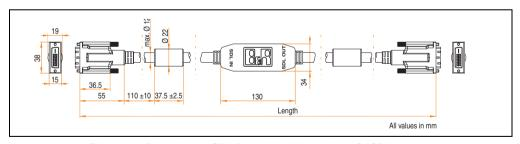
Figure 341: Dimensions - SDL flex cable with extender 5CASDL.0x00-13
