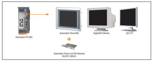
Figure 41: Monitor / Panel connection with DVI video signal
