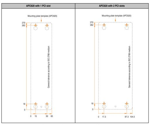
Table 136: Drilling templates - 1 and 2 PCI slots
