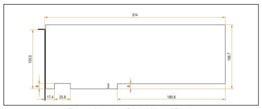
Figure 44: Dimensions - Standard full-size PCI cards
