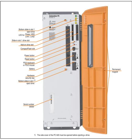
Figure 14: Interface overview - APC620, 3 PCI slot variant (front)
