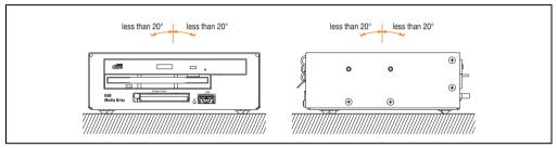
Figure 306: Mounting orientation of USB Media Drive 5MD900.USB2-00
