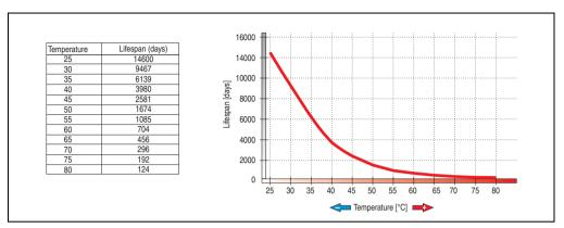
Figure 354: Temperature life span diagram
