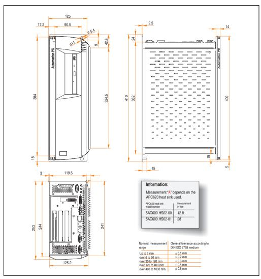
Figure 15: Dimensions - APC620, 3 PCI slot variant
