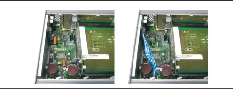
Figure 430: Plug in connection cable
