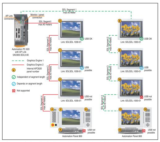
Figure 144: Configuration - Six AP900 and two AP800 devices via SDL (onboard) and SDL (AP Link)
