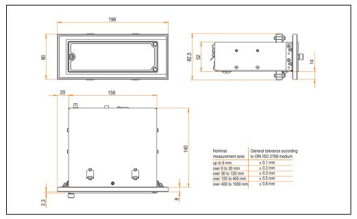
Figure 304: Dimensions - USB Media Drive with front cover
