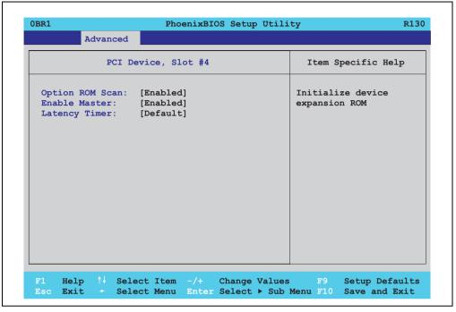
Figure 201: 855GME (ETX) - PCI device, slot #4
