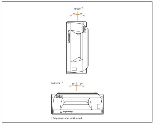
Figure 131: Mounting orientations for an APC620 with a slide-in DVD-R/RW / DVD+R/RW drive
