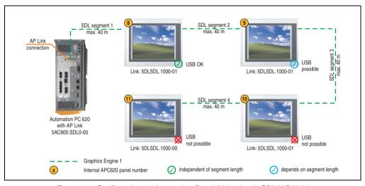
Figure 141: Configuration - 4 Automation Panel 900 units via SDL (AP Link)
