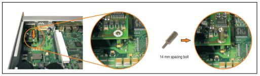
Figure 421: Screw in spacing bolt
