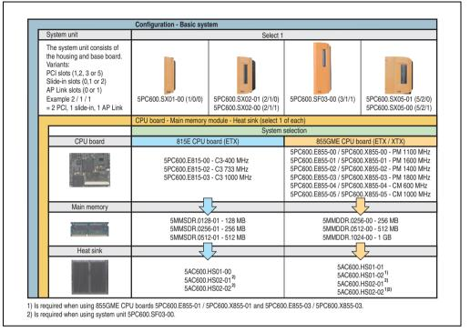
Figure 4: Selection guide - APC620 basic system with 1, 2, 3, and 5 PCI slots
