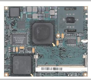
Figure 59: CPU boards 815E (ETX)
