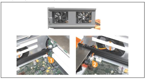
Figure 380: APC620 2PCI slots - Fan cable connection to the main board
