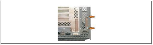
Figure 432: Remove UPS module cover
