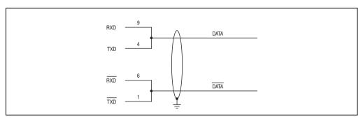
Figure 114: Add-on RS232/422/485 interface - operated in RS485 mode
