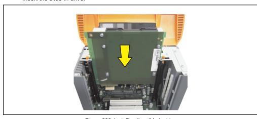
Figure 396: Installing the slide-in drive
