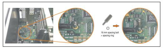
Figure 415: Screw in spacing bolt and spacing ring
