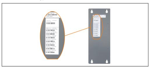
Figure 48: APC620 serial number sticker on back-side
