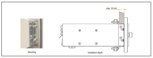
Figure 309: Front cover mounting and installation depth
