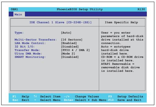
Figure 194: 855GME (ETX) IDE channel 1 slave setup
