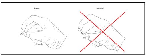
Figure 369: Battery handling
