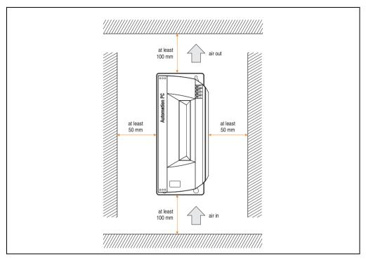
Figure 125: Air circulation spacing - Standard
