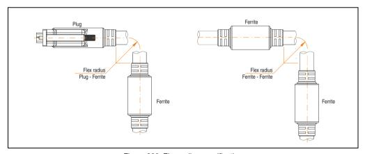
Figure 326: Flex radius specification
