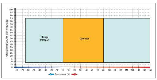
Figure 289: Temperature humidity diagram - CompactFlash cards 5CFCRD.xxxx-04
