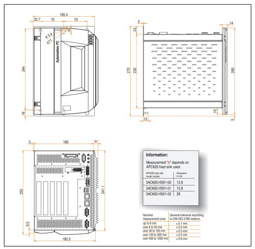
Figure 18: Dimensions - APC620, 5 PCI slot variant
