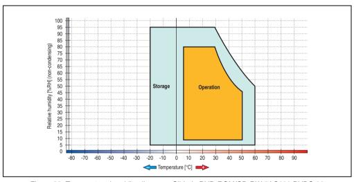
Figure 82: Temperature humidity diagram - Slide-in DVD-ROM/CD-RW 5AC600.DVDS-00
