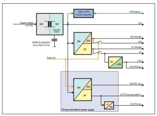
Figure 31: Supply voltage block diagram 3 PCI slots
