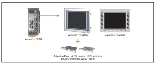
Figure 42: Monitor / Panel connection with SDL video signal
