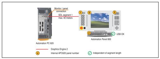
Figure 137: Configuration - An Automation Panel 800 via SDL (onboard)
