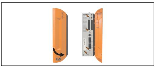
Figure 371: APC620 1PCI slot - Remove screws to install/ remove filter kit
