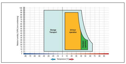
Figure 73: Temperature humidity diagram - Add-on hard disk 5AC600.HDDI-04
