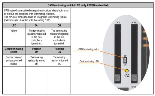
Table 37: CAN terminating switch / LED (only APC620 embedded)
