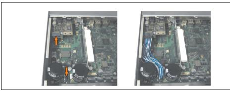
Figure 404: Plug in connection cable
