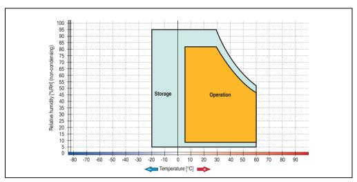
Figure 80: Temperature humidity diagram - Slide-in CD-ROM 5AC600.CDXS-00
