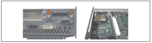
Figure 422: Install UPS module
