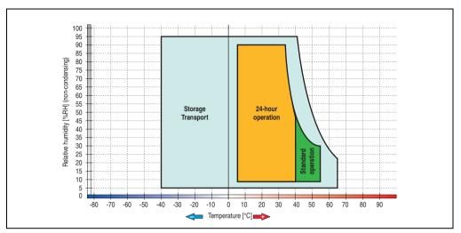
Figure 71: Temperature humidity diagram - Add-on hard disk 5AC600.HDDI-03
