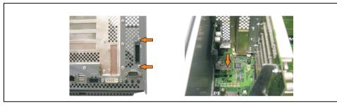
Figure 436: Install UPS module
