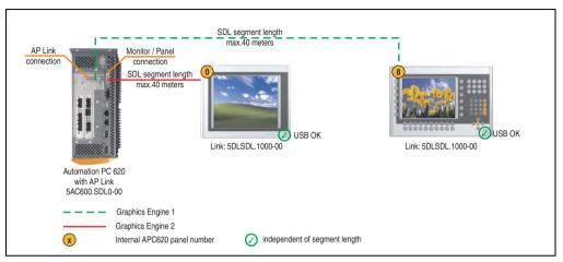
Figure 142: Configuration - Two Automation Panel 900 units via SDL (onboard) and SDL (AP Link)
