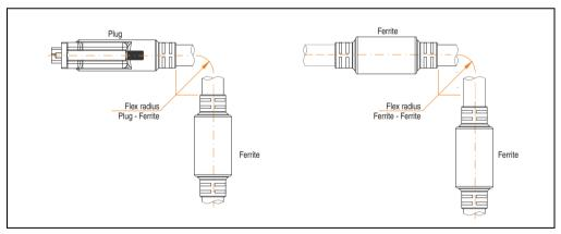
Figure 329: Flex radius specification
