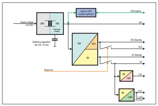
Figure 27: Supply voltage for the 5PC600.SX01-00 revision >= I0
