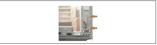
Figure 413: Remove UPS module cover
