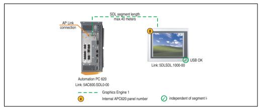
Figure 140: Configuration - One Automation Panel 900 via SDL (AP Link)
