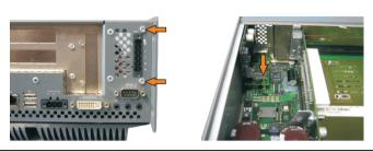
Figure 429: Install UPS module
