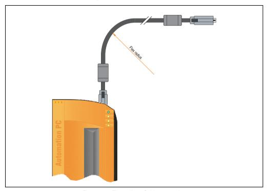
Figure 133: Flex radius - Cable connection
