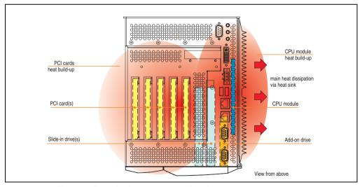
Figure 22: Example of worst-case conditions for temperature measurement
