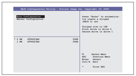
Figure 149: RAID Configuration Utility - Create RAID set - Striped
