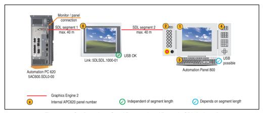
Figure 138: Configuration - One AP900 and an AP800 via SDL (onboard)
