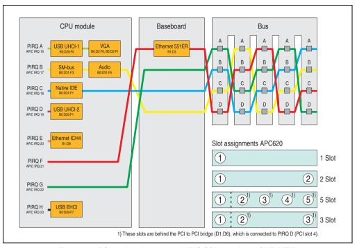
Figure 249: PCI routing with activated APIC CPU boards 855GME (XTX)
