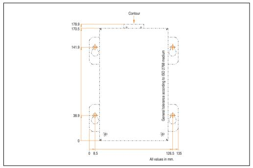
Figure 357: Drilling template for the battery unit
