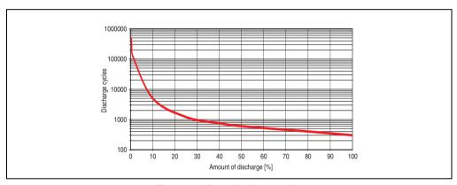
Figure 355: Deep discharge cycles
