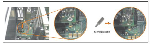
Figure 434: Screw in spacing bolt
