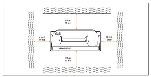
Figure 127: Optional circulation spacing
