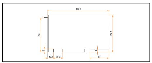
Figure 43: Dimensions - Standard half-size PCI cards
