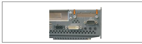
Figure 420: Remove UPS module cover
