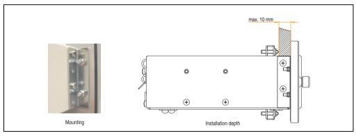
Figure 317: Front cover mounting and installation depth
