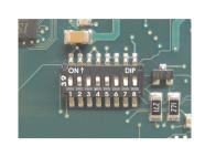
Figure 187: DIP switch on system unit
