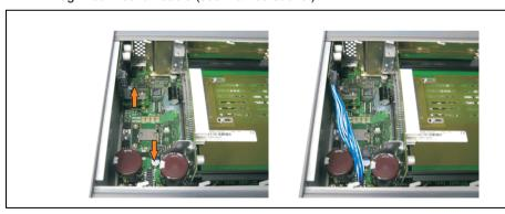
Figure 411: Plug in connection cable
