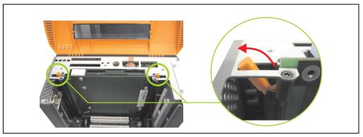
Figure 397: Release the slide-in slot releasing mechanisms
