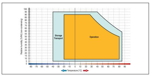
Figure 67: Temperature humidity diagram - Add-on hard disk 5AC600.HDDI-01
