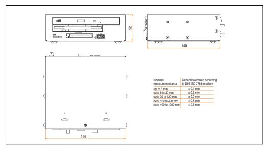
Figure 303: Dimensions for USB Media Drive 5MD900.USB2-00
