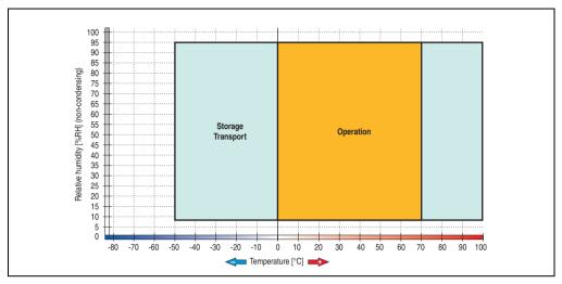
Figure 293: Temperature humidity diagram - CompactFlash cards 5CFCRD.xxxx-03
