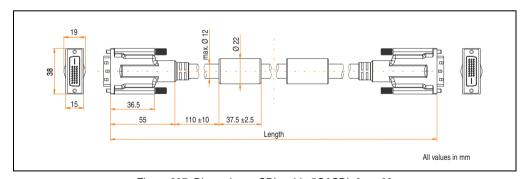
Figure 337: Dimensions - SDL cable 5CASDL.0xxx-03
