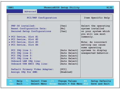
Figure 197: 815GME (ETX) - PCI/PNP configuration
