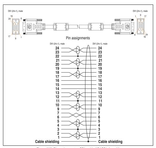
Figure 327: Pin assignments - SDL cable 5CASDL.0xxx-00
