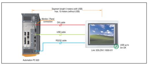
Figure 135: Configuration - One Automation Panel 900 via DVI (onboard)
