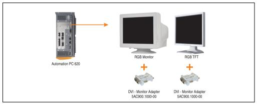
Figure 40: Monitor / Panel connection with RGB video signal
