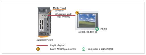
Figure 136: Configuration - An Automation Panel 900 via SDL (onboard)
