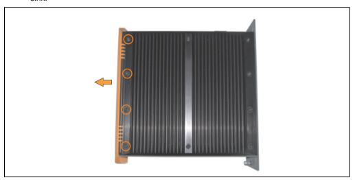
Figure 445: Removing the APC620 front cover
