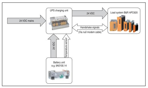
Figure 359: Block diagram of the UPS
