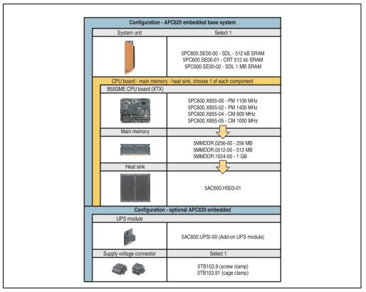
Figure 6: Selection guide - Basic system and optional components APC620 embedded
