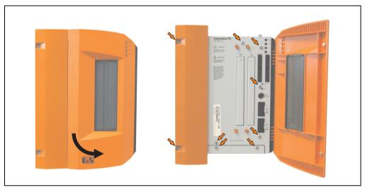
Figure 388: APC620 5PCI slot - Remove screws to install/ remove filter kit
