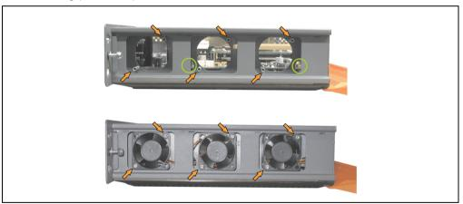
Figure 374: APC620 1PCI slot - Fan installation
