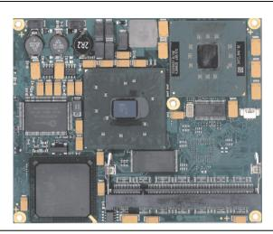
Figure 60: CPU boards 855GME (ETX)
