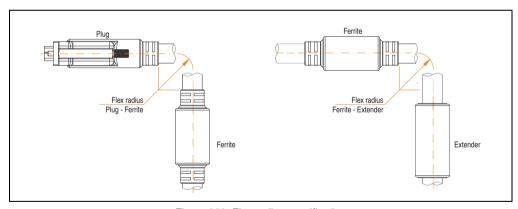
Figure 332: Flex radius specification
