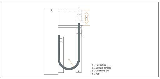
Figure 287: Test structure - Cable drag chain
