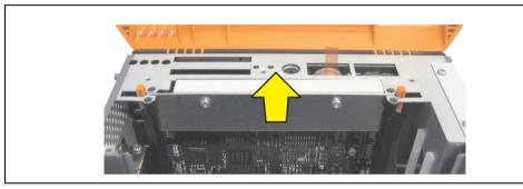
Figure 395: Removing the slide-in dummy module
