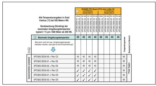
Figure 26: Ambient temperatures for embedded systems with an 855GME CPU board (EXT / XTX)
