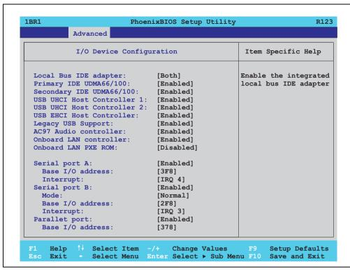
Figure 173: 815E (ETX) I/O Device Configuration
