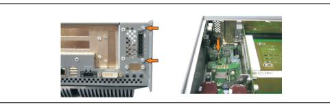
Figure 410: Install UPS module
