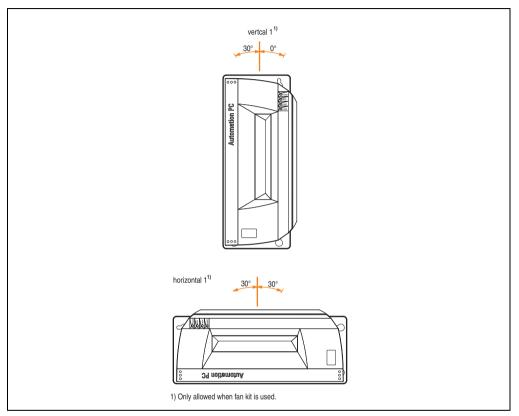
Figure 130: Mounting orientations for an APC620 with a slide-in DVD-ROM/CD-RW drive
