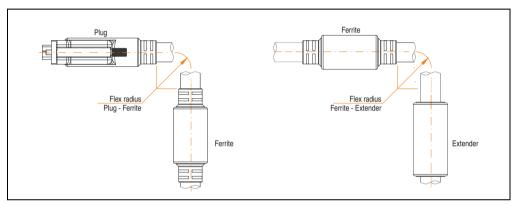
Figure 340: Flex radius specification
