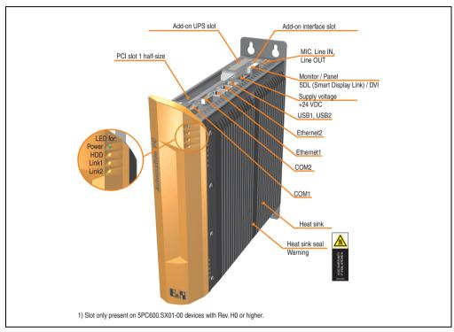
Figure 7: Interface overview - APC620, 1 PCI slot variant (top)
