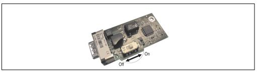
Figure 111: Terminating resistor - Add-on CAN interface 5AC600.CANI-00
