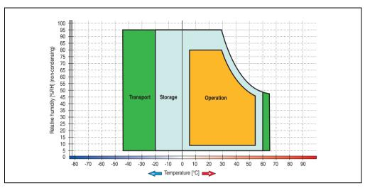
Figure 84: Temperature humidity diagram - Slide-in DVD-R/RW, DVD+R/RW 5AC600.DVRS-00
