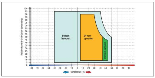
Figure 89: Temperature humidity diagram - Slide-in hard disk 5AC600.HDDS-00
