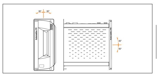
Figure 126: Mounting orientation - Optional
