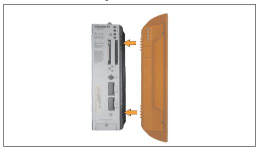
Figure 449: Attaching the front cover
