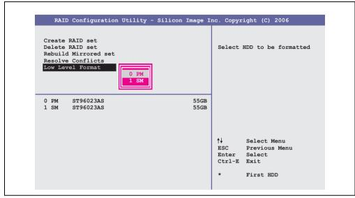
Figure 154: RAID Configuration Utility - Low level format
