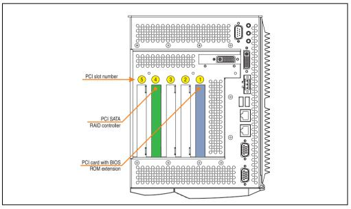
Figure 107: PCI slot numbering on APC620 systems with 5 PCI slots
