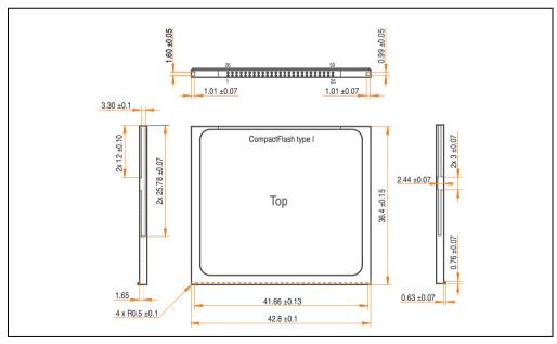
Figure 290: Dimensions - CompactFlash card Type I
