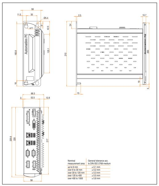
Figure 21: APC620 embedded variant - dimensions
