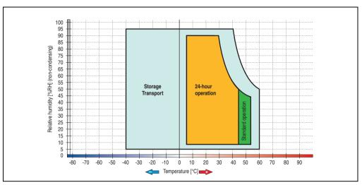
Figure 65: Temperature humidity diagram - Add-on hard disk 5AC600.HDDI-00
