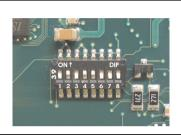
Figure 247: DIP switch on system unit
