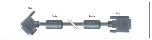
Figure 328: SDL cable with 45° plug (similar)
