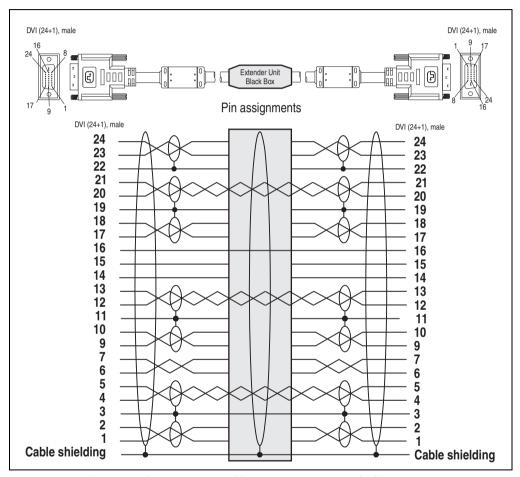
Figure 334: Pin assignments - SDL cable with extender 5CASDL.0x00-10
