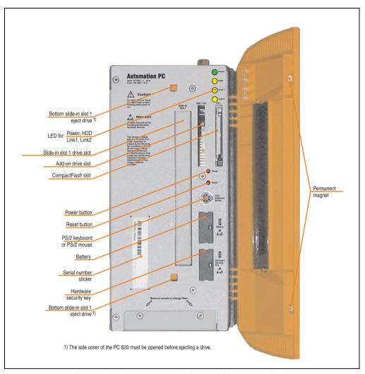
Figure 11: Interface overview - APC620, 2 PCI slot variant (front)
