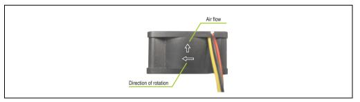
Figure 373: Markings for direction of airflow / fan rotation
