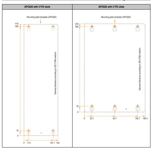
Table 137: Drilling templates - 3 and 5 PCI slots
