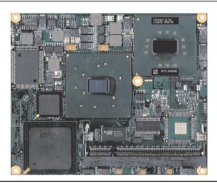
Figure 61: CPU boards 855GME (XTX)
