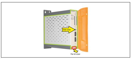
Figure 372: APC620 1PCI slot - Remove side cover and fan kit cover
