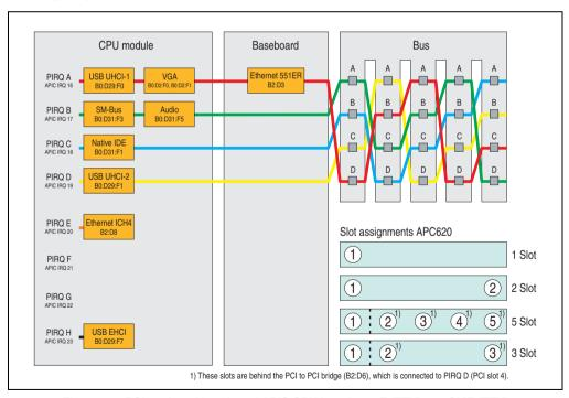
Figure 248: PCI routing with activated APIC CPU boards 815E (ETX), 855GME (ETX)
