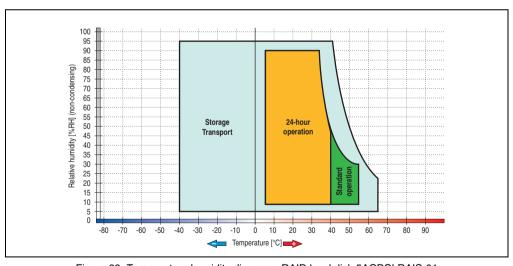
Figure 99: Temperature humidity diagram - RAID hard disk 5ACPCI.RAIS-01
