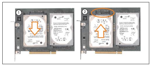
Figure 444: Hard disk exchange
