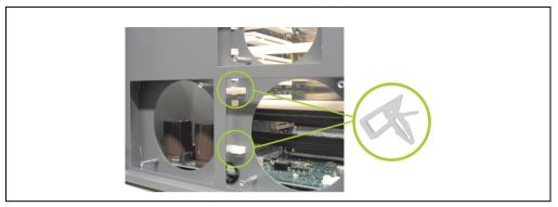
Figure 390: APC620 5PCI attach cable fasteners
