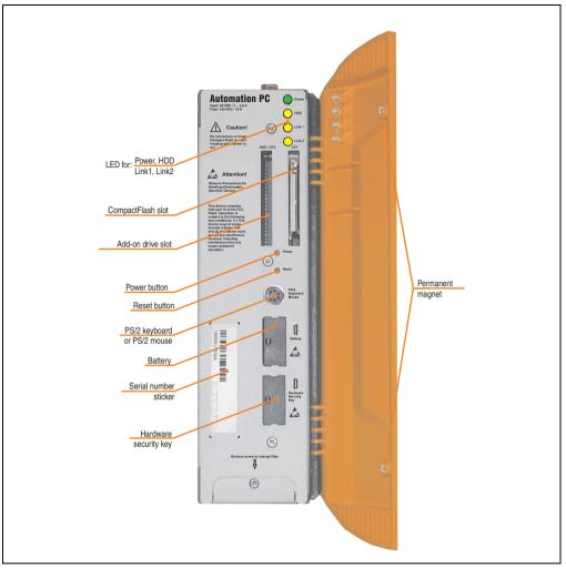
Figure 8: Interface overview - APC620, 1 PCI slot variant (front)
