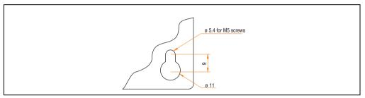
Figure 123: Mounting plates for the APC620
