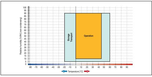
Figure 318: Temperature humidity diagram for flash drives 5MMUSB.xxxx-00
