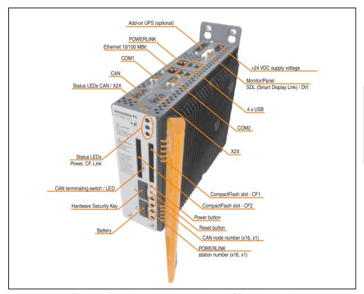
Figure 36: General device interfaces example - APC620 embedded
