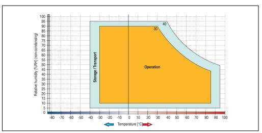
Figure 77: Temperature humidity diagram - Add-on hard disk 5AC600.HDDI-06
