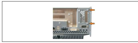
Figure 425: Remove UPS module cover
