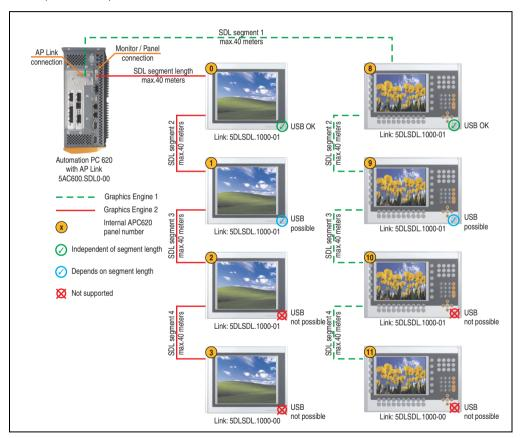
Figure 143: Configuration - Eight Automation Panel 900 units via SDL (onboard) and SDL (AP Link)
