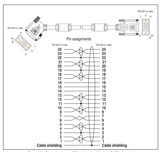
Figure 330: Pin assignments - SDL cable with 45° plug 5CASDL.0xxx-01
