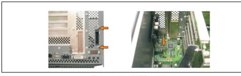
Figure 417: Install UPS module
