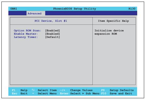
Figure 198: 855GME (ETX) - PCI device, slot #1
