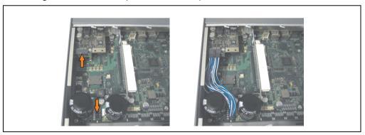
Figure 423: Plug in connection cable
