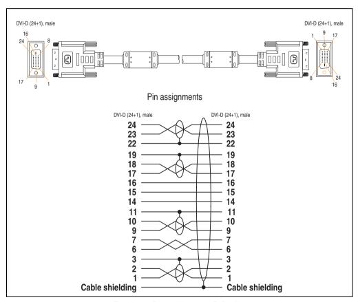
Figure 324: Pin assignments - DVI cable
