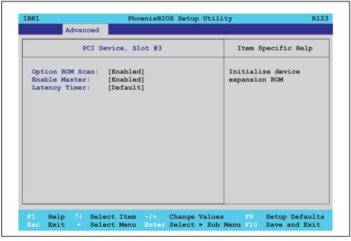
Figure 170: 815E (ETX) PCI device, slot #3
