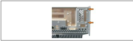
Figure 406: Remove UPS module cover
