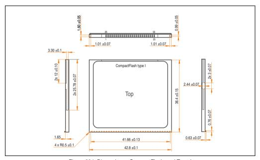
Figure 294: Dimensions - CompactFlash card Type I
