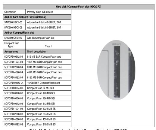
Table 65: Technical data - Hard disk / CompactFlash slot (HDD/CF2)
