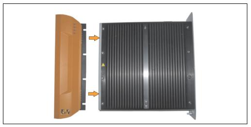
Figure 446: Mounting the APC620 front cover
