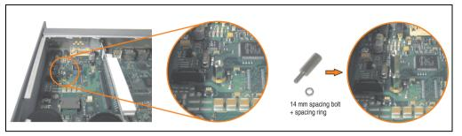
Figure 402: Screw in spacing bolt and spacing ring
