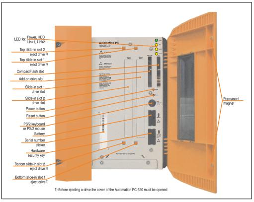
Figure 17: Interface overview - APC620, 5 PCI slot variant (front)
