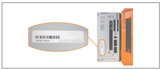
Figure 47: APC620 serial number sticker on front-side
