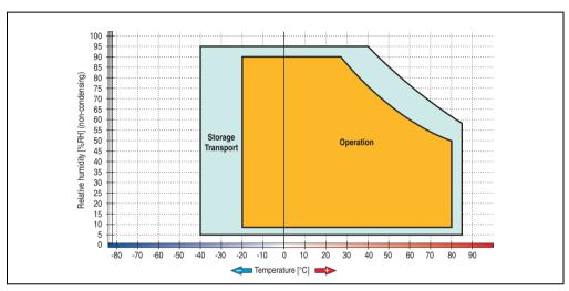
Figure 91: Temperature humidity diagram - Slide-in hard disk 5AC600.HDDS-01
