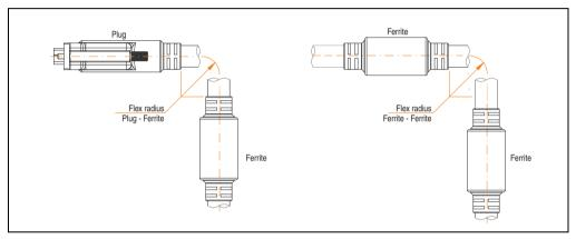
Figure 336: Flex radius specification
