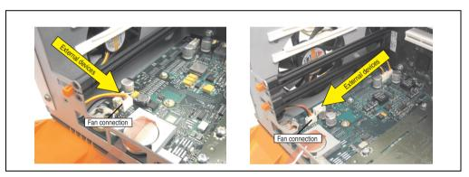
Figure 451: Connector location for external devices
