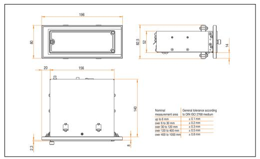
Figure 312: Dimensions - USB Media Drive with front cover
