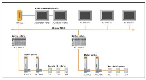
Figure 2: APC620 as visualization device
