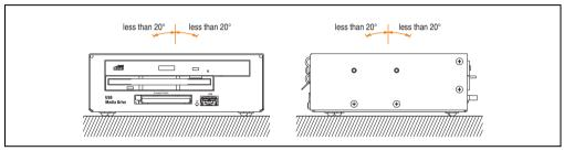
Figure 314: Mounting orientation - 5MD900.USB2-01
