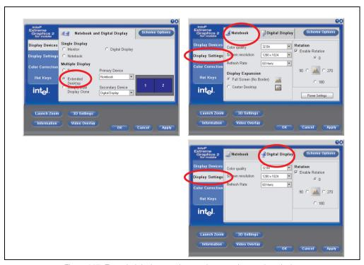
Figure 267: Extended desktop settings - primary and secondary device
