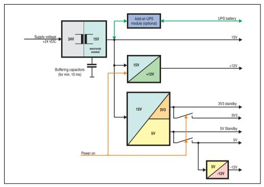
Figure 28: Supply voltage for the 5PC600.SX01-00 revision < I0
