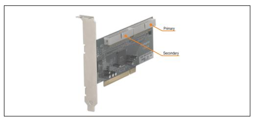
Figure 95: RAID controller - 5ACPCI.RAIC-00
