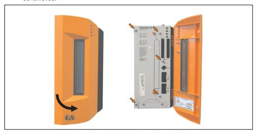
Figure 440: Mounting the side cover - APC620, 2 PCI slot
