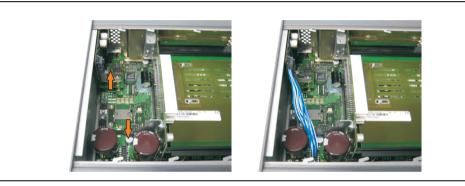
Figure 430: Plug in connection cable
