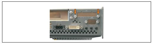
Figure 401: Remove UPS module cover
