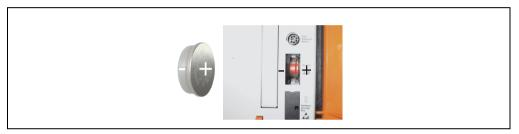
Figure 370: Battery polarity
