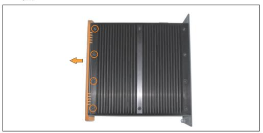
Figure 445: Removing the APC620 front cover
