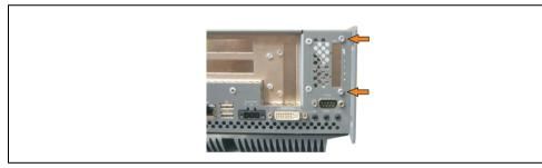
Figure 425: Remove UPS module cover
