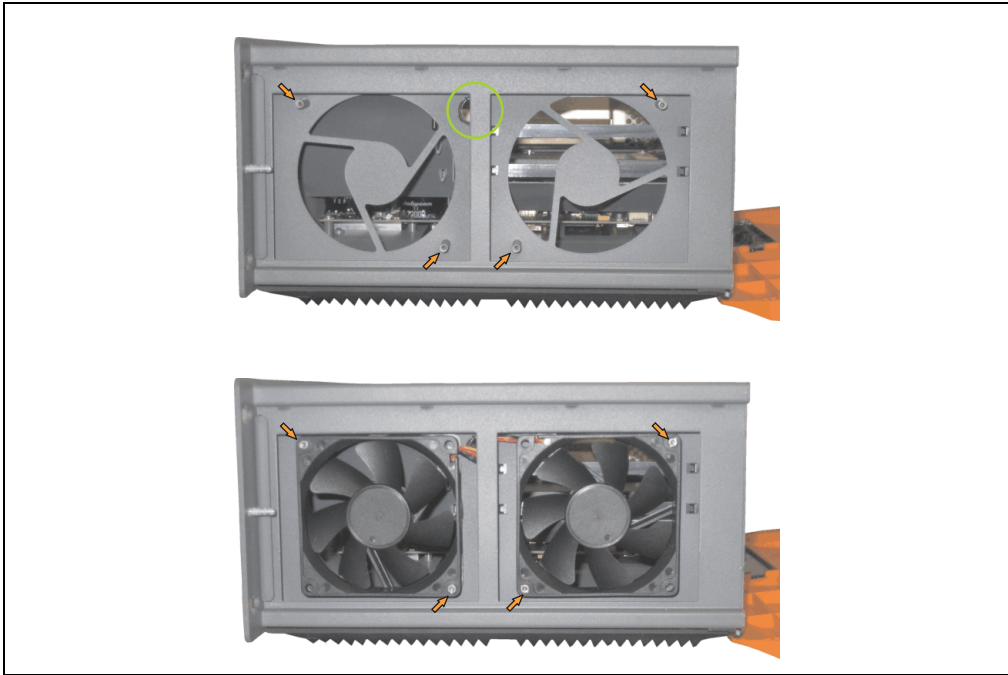
Figure 385: APC620 3PCI slot - Fan installation
