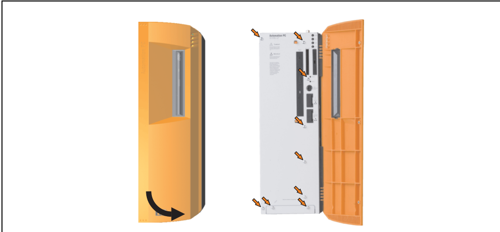
Figure 382: APC620 3PCI slot - Remove screws to install/ remove filter kit
