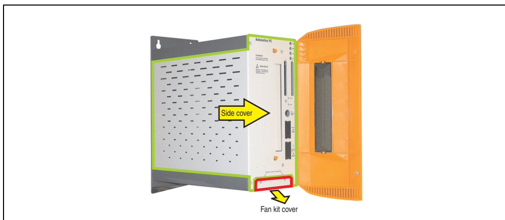
Figure 377: APC620 2PCI slots - Remove side cover and fan kit cover
