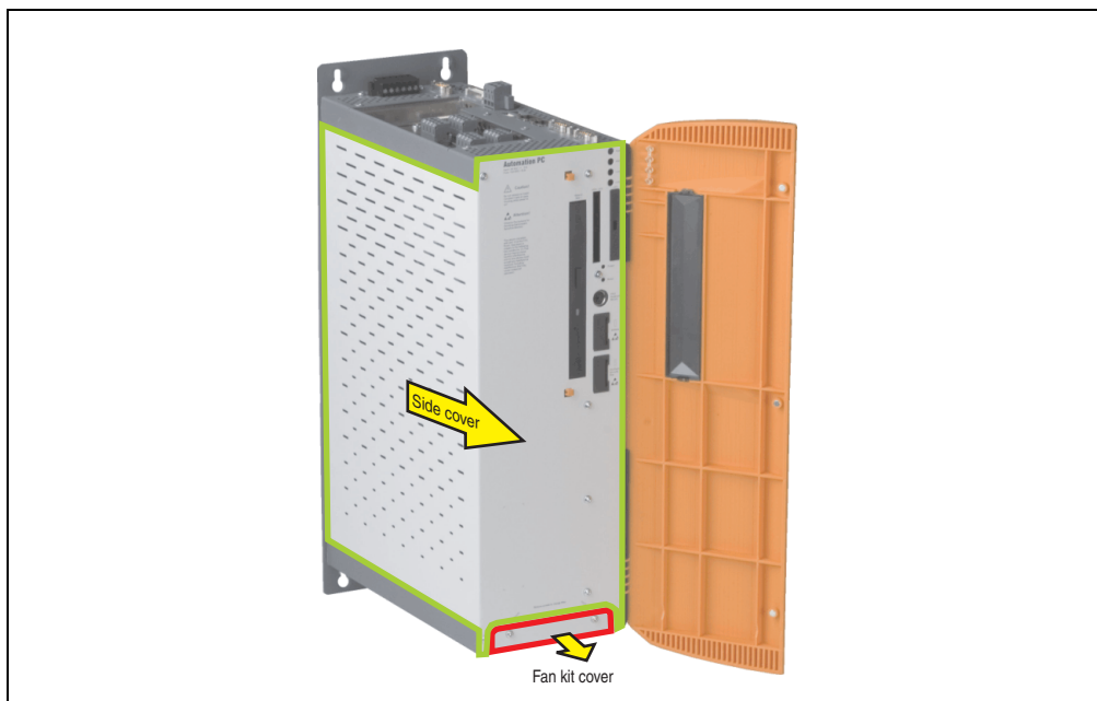
Figure 383: APC620 3PCI slots - Remove side cover and fan kit cover
