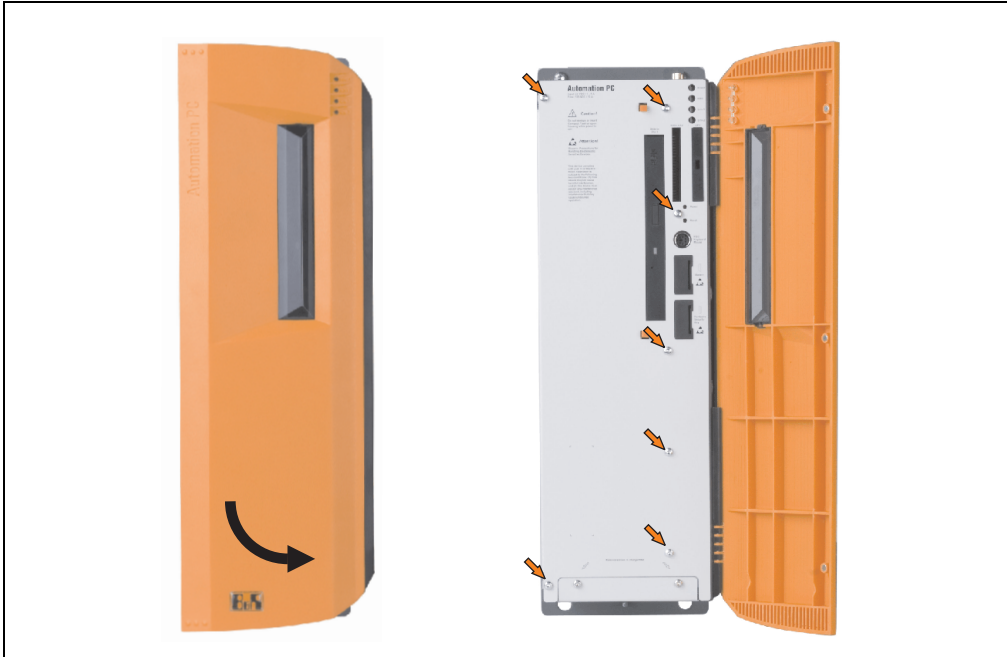
Figure 441: Mounting the side cover - APC620, 3 PCI slot
