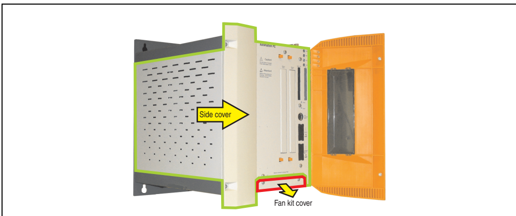
Figure 389: APC620 5PCI slot - Remove side cover and fan kit cover
