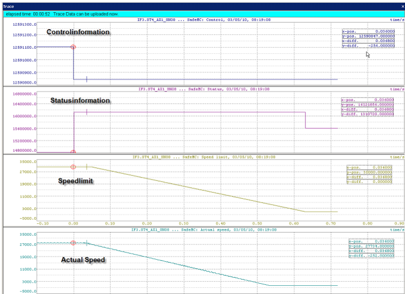
Figure 37: ACOPOSMulti trace of available SafeMC data
