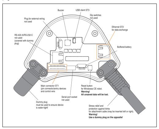
Figure 37: Attachment shaft
