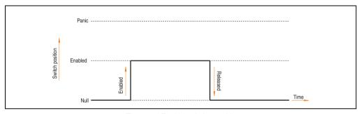
Figure 19: Enable switch - enable
