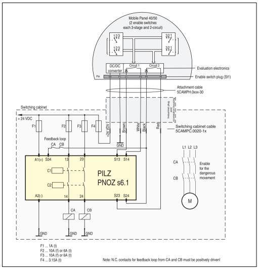
Figure 42: Connection example - Enable switch
