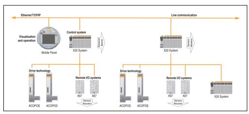
Figure 2: Mobile operation and monitoring
