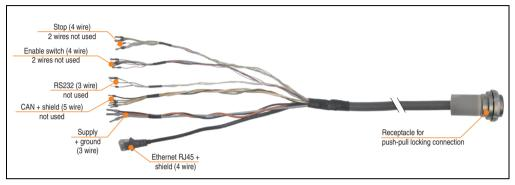
Figure 29: Mobile Panel switching cabinet cable 5CAMPC.0020-10
