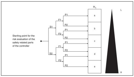
Figure 58: Risk diagram to determine the PL<sub>r</sub> for every safety function
