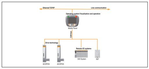
Figure 1: Mobile control and visualization
