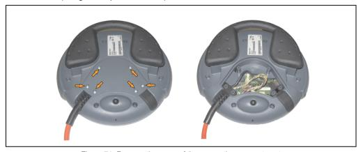
Figure 71: Remove the cover of the connection compartment
