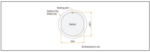
Figure 34: Drilling template - Receptacle
