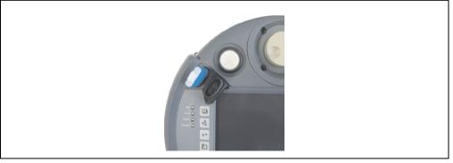
Figure 44: USB interface - insert flash drive
