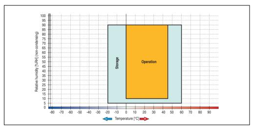
Figure 62: Temperature humidity diagram - USB flash drive - 5MMUSB.xxxx-00
