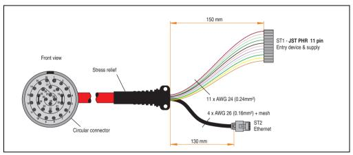
Figure 28: Cable specifications - Attachment cable 5CAMPH.0xxx-30
