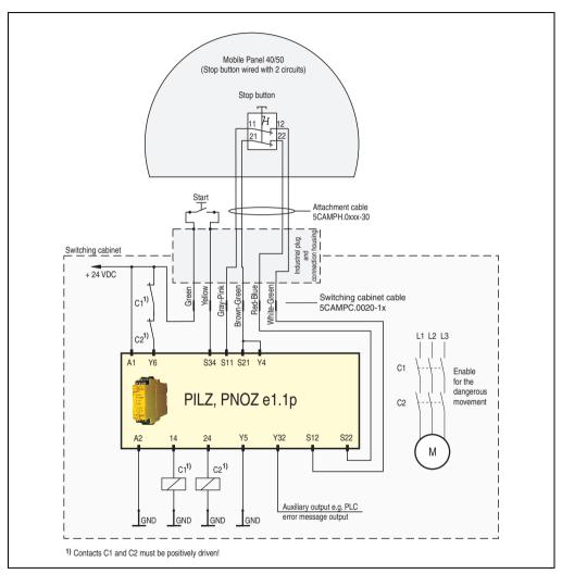
Figure 41: Connection example for stop button
