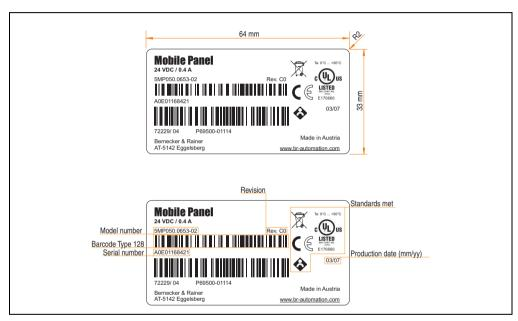
Figure 11: Design / dimensions - Type plate
