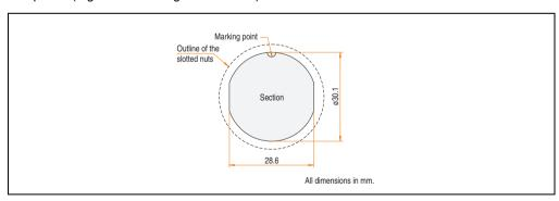
Figure 31: Drilling template - Receptacle
