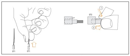
Figure 38: Removing ST1 and ST2
