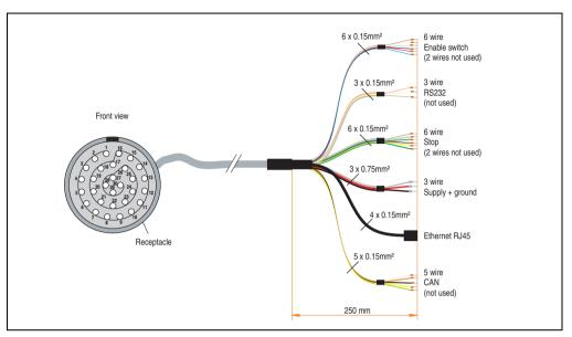
Figure 30: Cable layout - switching cabinet cable 5CAMPC.0020-10
