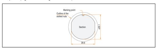
Figure 31: Drilling template - Receptacle
