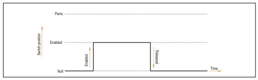
Figure 19: Enable switch - enable
