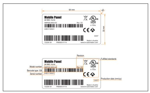
Figure 11: Design / dimensions - Serial number sticker
