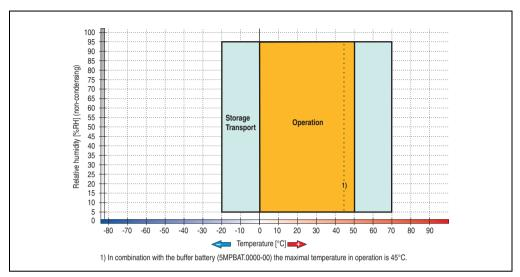
Figure 10: Temperature humidity diagram
