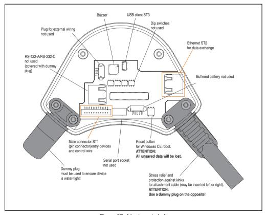
Figure 37: Attachment shaft
