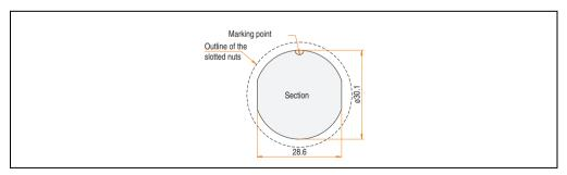
Figure 34: Drilling template - Receptacle
