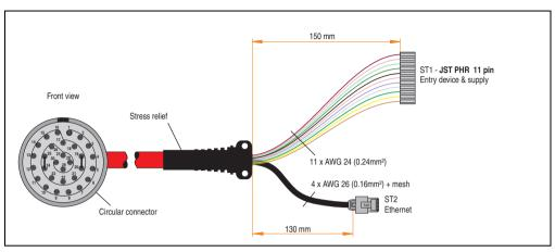
Figure 28: Attachment cable specifications 5CAMPH.0xxx-30
