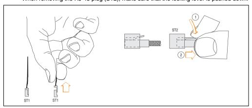
Figure 38: Removing ST1 and ST2
