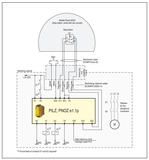
Figure 42: Connection example - Enable switch
