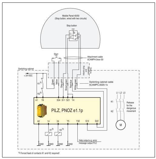
Figure 41: Connection example for stop button
