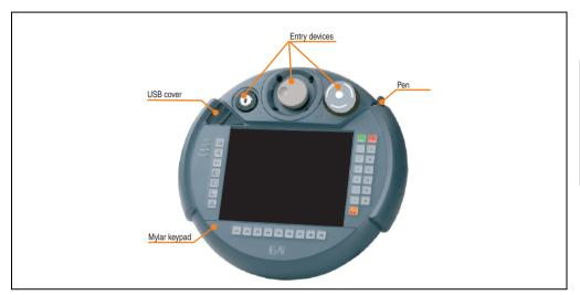
Figure 13: Mobile Panel operating unit
