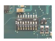
Figure 236: DIP switch on system unit
