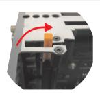
Figure 383: Slide-in slot releasing mechanism start position
