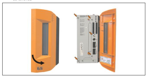
Figure 424: Mounting the side cover - APC620, 2 PCI slot
