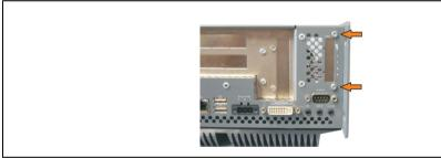
Figure 409: Remove UPS module cover
