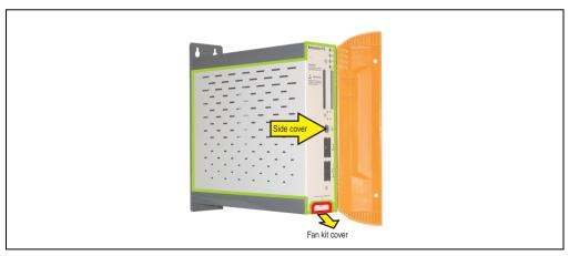
Figure 356: APC620 1PCI slot - Remove side cover and fan kit cover
