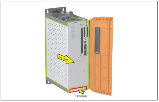
Figure 367: APC620 3PCI slots - Remove side cover and fan kit cover
