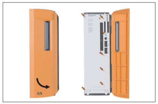
Figure 425: Mounting the side cover - APC620, 3 PCI slot
