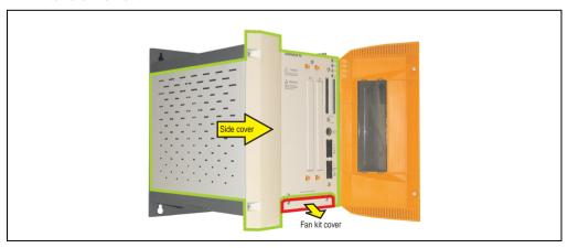
Figure 373: APC620 5PCI slot - Remove side cover and fan kit cover
