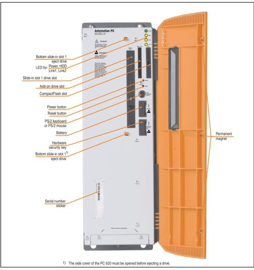
Figure 12: Interface overview - APC620, 3 PCI slot variant (front)
