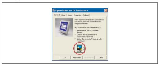
Figure 262: Touch screen calibration
