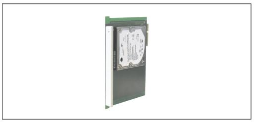
Figure 84: Slide-in hard disk 40 GB - 5AC600.HDDS-02
