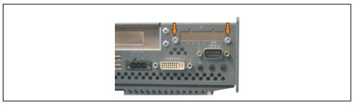
Figure 404: Remove UPS module cover
