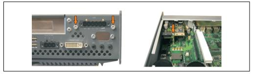
Figure 387: Install UPS module
