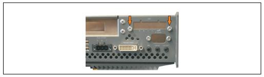
Figure 385: Remove UPS module cover
