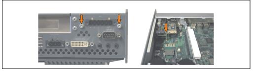
Figure 406: Install UPS module
