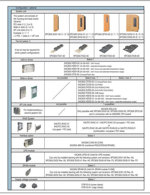
Figure 3: Selection guide - APC620 optional components with 1, 2, 3, and 5 PCI slots
