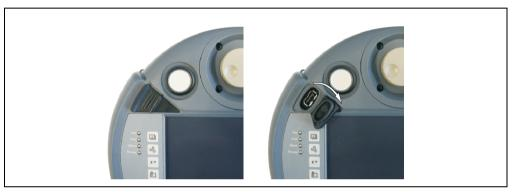
Figure 39: USB interface - open protective cap
