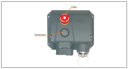
Figure 56: Connection box 4MPCBX.0000-00
