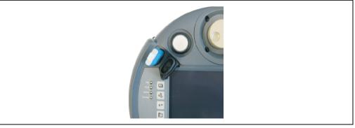
Figure 40: USB interface - insert flash drive
