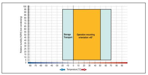
Figure 6: Temperature humidity diagram
