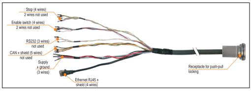
Figure 28: Mobile Panel switching cabinet cable - 5CAMPC.0020-11
