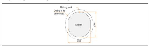
Figure 27: Drilling template - receptacle
