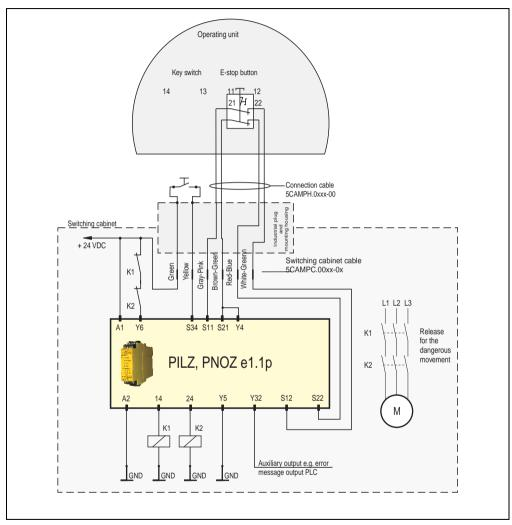
Figure 37: Connection example for stop button
