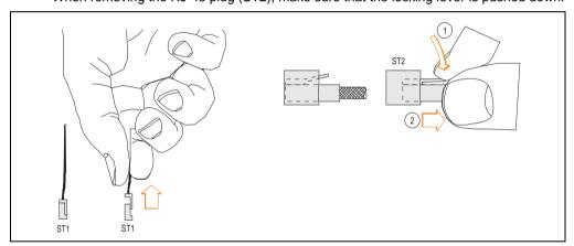
Figure 34: Removing ST1 and ST2
