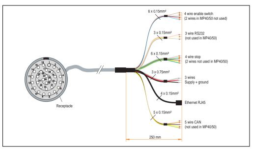
Figure 29: Cable layout - Switching cabinet cable - 5CAMPC.0020-11
