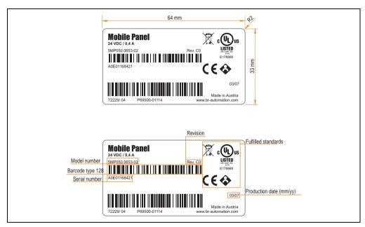
Figure 7: Design/dimensions - Serial number sticker
