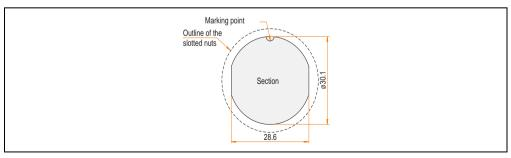
Figure 30: Drilling template - Receptacle
