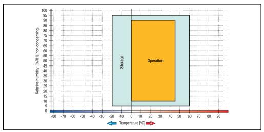
Figure 50: Temperature humidity diagram - USB flash drive - 5MMUSB.xxxx-00
