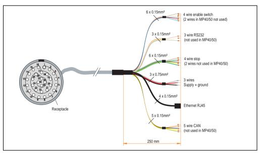
Figure 26: Cable layout - switching cabinet cable - 5CAMPC.0020-10
