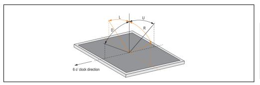
Figure 57: Viewing angle definition
