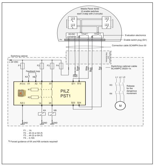
Figure 38: Connection example - enable switch
