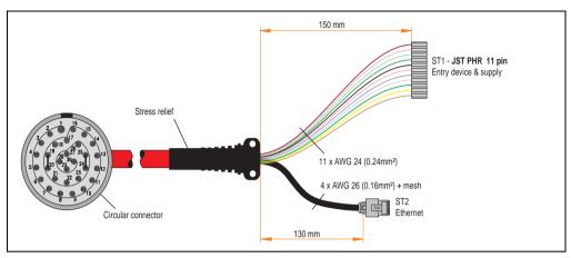
Figure 24: Attachment cable specifications - 5CAMPH.0xxx-30
