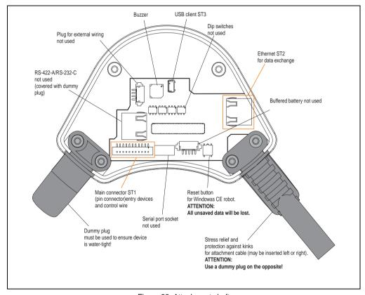
Figure 33: Attachment shaft
