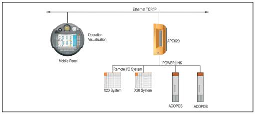
Figure 42: Mobile thin client
