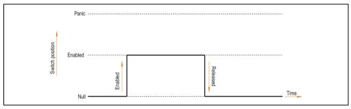
Figure 15: Enable switch - Enable
