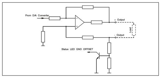
Figure 200: NC150 output diagram for analog outputs
