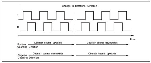
Figure 202: NC150 counting direction in operation mode positioning
