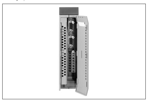
Figure 197: NC150 operational and connection elements
