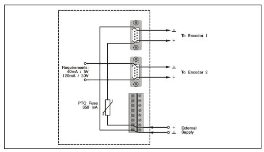
Figure 198: NC150 encoder supply
