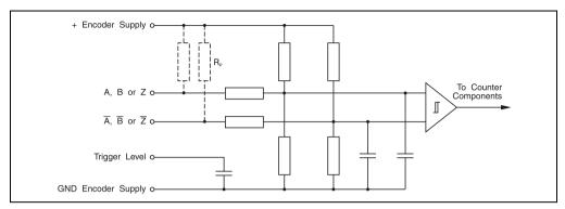
Figure 201: NC150 input circuit for counter inputs
