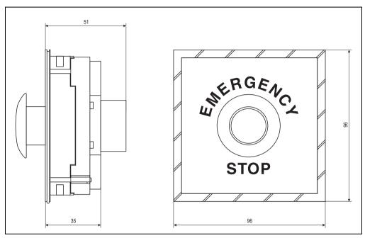
Figure 194: Dimensions - keypad module with E-stop button
