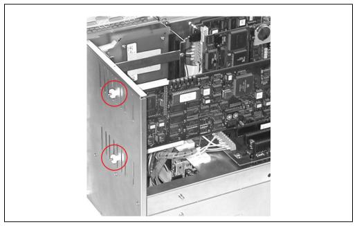
Figure 84: Fasteners for full-size cards
