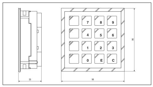
Figure 190: Dimensions - keypad module with 12+4 keys
