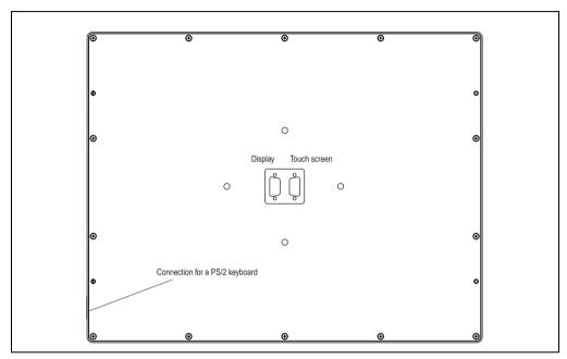
Figure 160: Connections - 5D5212.04 revision >= G0
