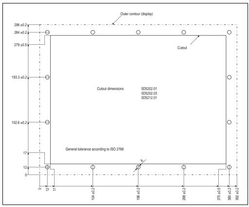
Figure 150: Cutout installation - 5D5202.01, 5D5202.03 and 5D5212.01
