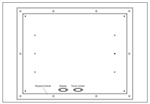
Figure 142: Connections - 5D5201.03 and 5D5211.03
