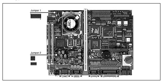
Figure 57: Jumper settings on mainboards with Socket 7 (ZIF)
