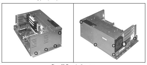
Figure 50: Removing the screws
