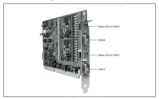
Figure 260: RS232 interface board
