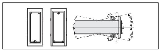
Figure 276: Mounting guidelines - controller R-IDE CD-ROM/LS120 drive (horizontal / vertical)
