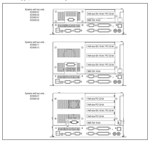
Figure 82: Slot assignments - PROVIT 5000 display units
