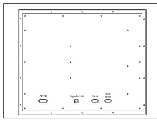
Figure 168: Connections - 5D5213.01 revision < F0
