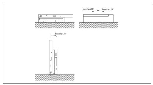
Figure 41: Mounting guidelines - 5A5600.05 controller
