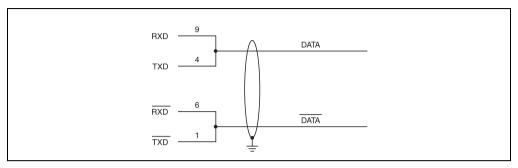
Figure 100: Operation of COM3 or COM4 interface in RS485 mode
