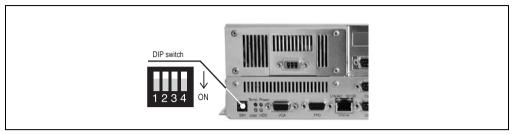
Figure 77: DIP switch for the IPC5000C and IPC5600C
