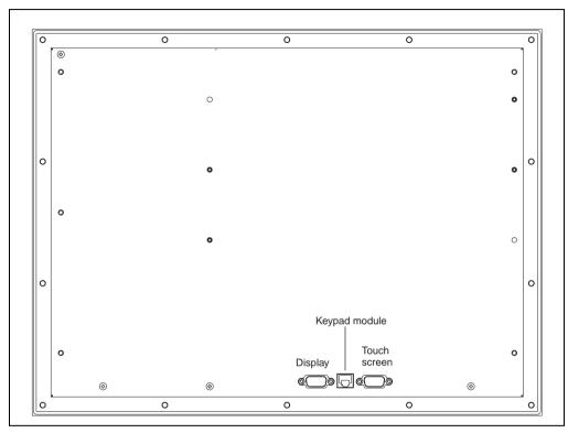
Figure 156: Connections - 5D5212.02 revision >= I0
