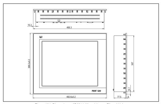
Figure 164: Dimensions - 5D5211.03 revision >= F0 and higher
