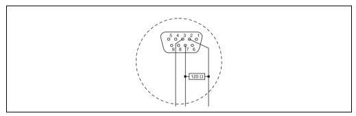
Figure 102: Terminating resistor connections for 9-pin DSUB plug
