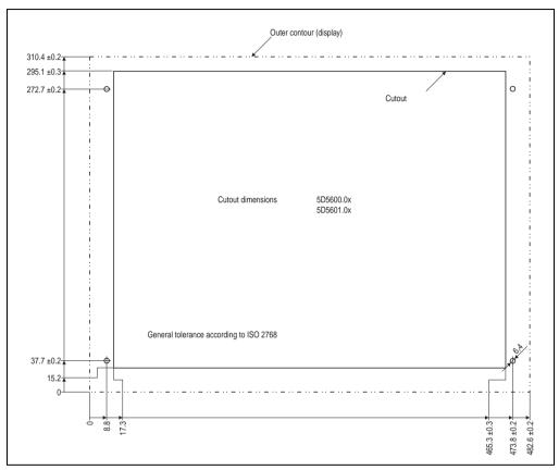
Figure 182: Cutout installation - 5D5600.0x and 5D5601.0x
