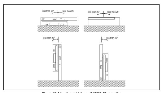
Figure 43: Mounting guidelines - 5A5600.07 controller
