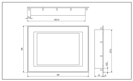
Figure 149: Dimensions - 5D5202.01, 5D5202.03 and 5D5212.01
