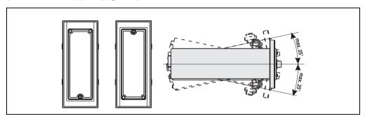
Figure 272: Mounting guidelines - controller R-IDE CD-ROM/LS120 drive (horizontal / vertical)
