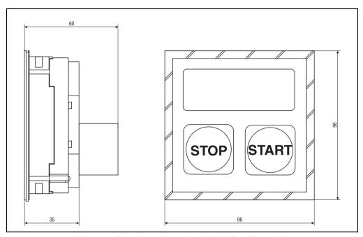
Figure 196: Dimensions - keypad module with Start/Stop switch
