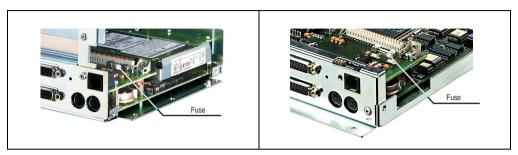
Figure 62: Fuse position for IPC5000 (left) and IPC5600 (right)
