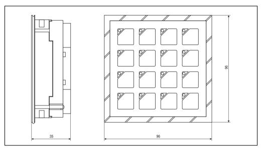
Figure 189: Dimensions - keypad module with 16 keys
