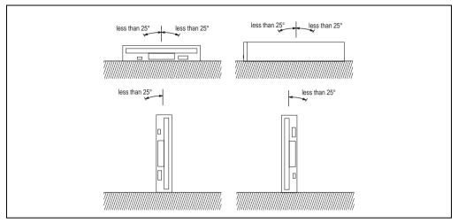
Figure 37: Mounting guidelines - 5A5600.03 controller
