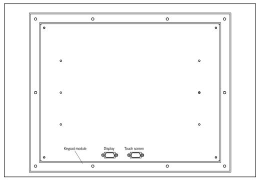
Figure 157: Connections - 5D5212.02 revision < I0
