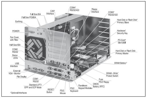
Figure 22: IPC5600 components (bus unit with 6 slots)
