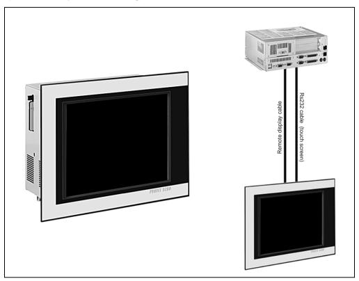
Figure 115: Standard mounting (left) and remote mounting (right)
