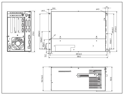
Figure 12: Dimensions - IPC5600 (4 slot design)
