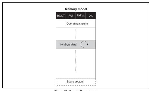
Figure 96: Ring buffer example
