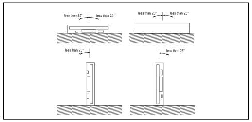
Figure 31: Mounting guidelines - 5A5600.01
