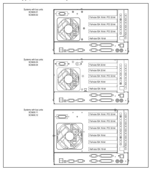
Figure 83: Slot assignments - PROVIT 5600 display units
