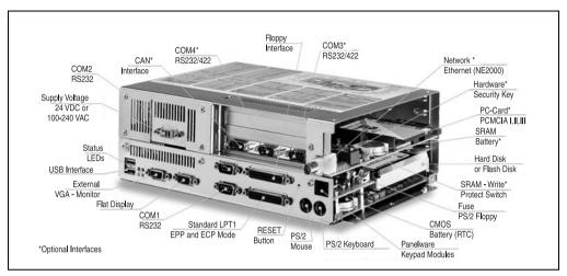
Figure 19: IPC5000 components (bus unit with 2 slots)
