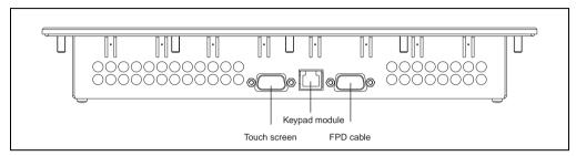
Figure 125: Connections - 5D5200.01 and 5D5210.01 revision >= G0
