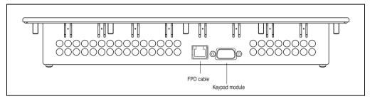
Figure 121: Connections - 5D5100.01 and 5D5100.04
