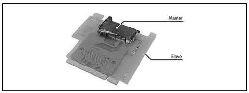
Figure 95: Silicon disk (CompactFlash card) on the adapter card
