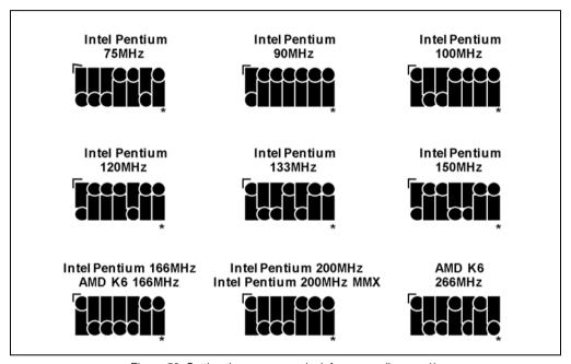
Figure 58: Setting the processor clock frequency (jumper 1):
