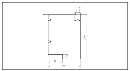
Figure 99: Interface board dimensions
