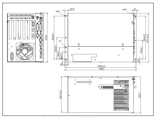
Figure 17: Dimensions - IPC5600C (6 slot design)
