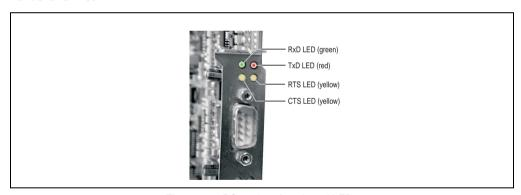
Figure 261: RS232 interface board LEDs
