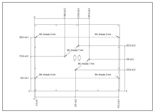
Figure 162: Flange drill holes - 5D5212.04 revision G0 and later
