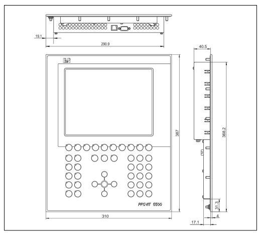
Figure 175: Dimensions - 5D5510 revision F0 and later
