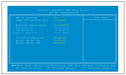
Figure 220: PnP/PCI configuration setup
