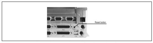
Figure 76: Reset button for the IPC5000C and IPC5600C
