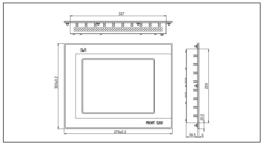
Figure 140: Dimensions - 5D5211.03 starting with revision J0
