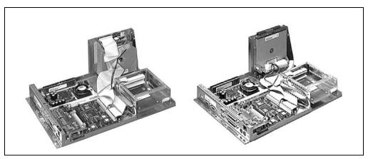
Figure 54: Aligning the drive to the front or the back
