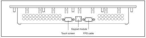
Figure 136: Connections - 5D5211.02 revision >= F0
