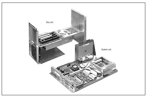
Figure 51: Detaching the bus unit
