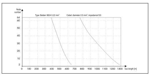
Figure 259: CAN - number of nodes / bus length
