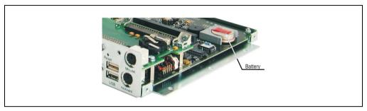
Figure 75: Battery holder for IPC5000C and IPC5600C
