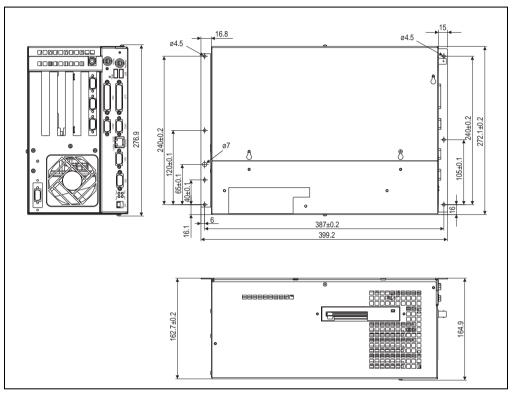
Figure 13: Dimensions - IPC5600C (4 slot design)
