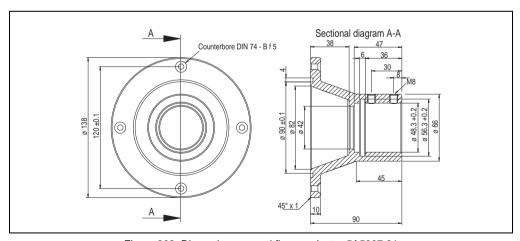
Figure 303: Dimensions - panel flange adapter 5A5007.01
