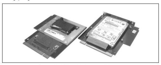
Figure 92: Hard disk - models 5A5001.13 and 5A5001.16
