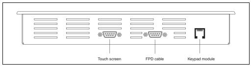
Figure 135: Connections - 5D5201.02 and 5D5211.02
