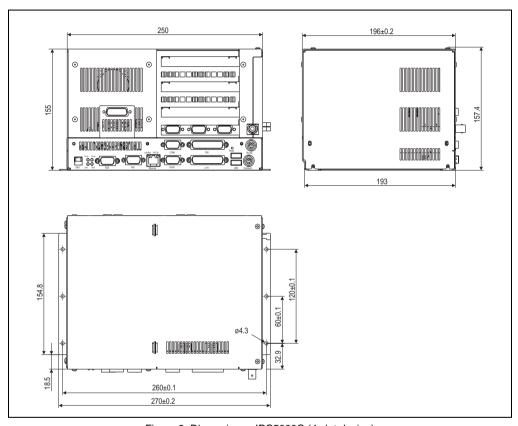
Figure 9: Dimensions - IPC5000C (4 slot design)
