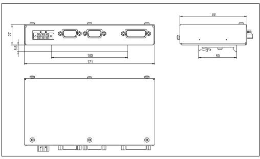
Figure 298: Dimensions - GS link remote unit 5A5010.02
