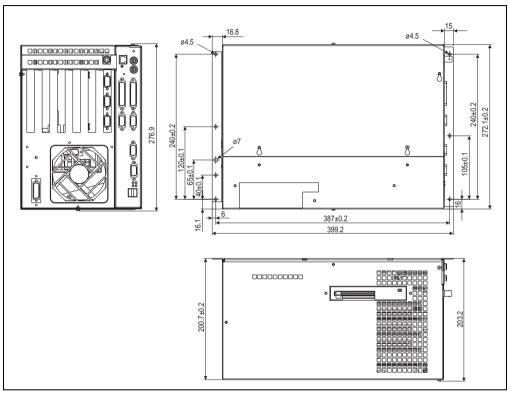
Figure 16: Dimensions - IPC5600 (6 slot design)
