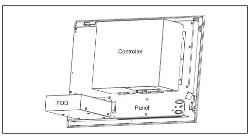
Figure 36: Mounting example of an FDD 5A5600.03 with controller on a panel
