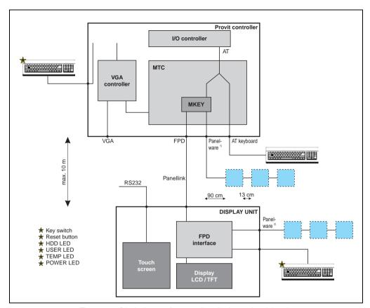
Figure 117: Block diagram for controller, display and peripherals
