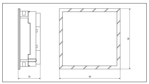
Figure 193: Dimensions - dummy module
