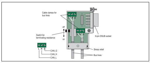
Figure 103: CAN bus connector 7AC911.9
