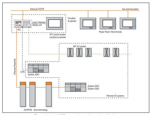
Figure 1: Industrial PC as central controller and visualization
