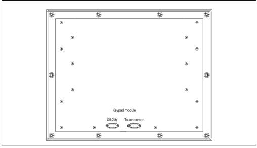
Figure 143: Connections - 5D5211.03 revision I0
