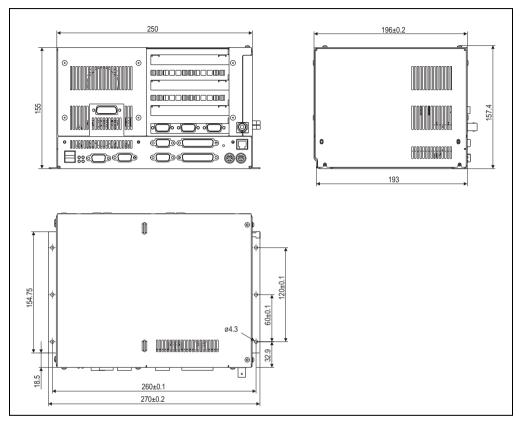
Figure 8: Dimensions - IPC5000 (4 slot design)
