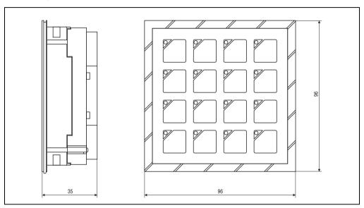
Figure 187: Dimensions - standard keypad modules
