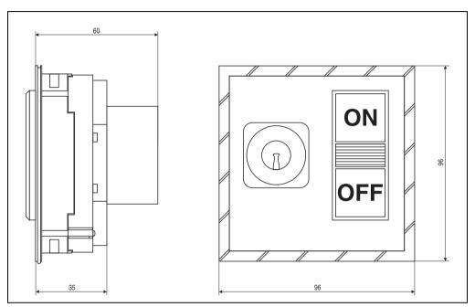
Figure 195: Dimensions - keypad module with key switch
