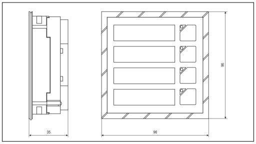
Figure 192: Dimensions - keypad module with 4 keys
