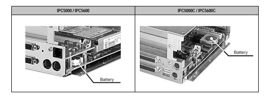
5) Remove the battery from the holder by pulling the removal strip (do not use uninsulated tools -> risk of short circuiting). The battery should not be held by its edges. **Insulated** tweezers may also be used for removing the battery.
