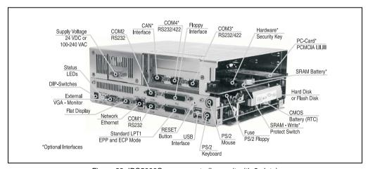
Figure 23: IPC5000C components (bus unit with 2 slots)
