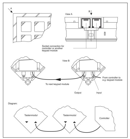
Figure 188: Connection to the controller or other keypad modules.
