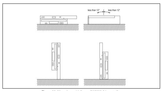
Figure 39: Mounting guidelines - 5A5600.04 controller
