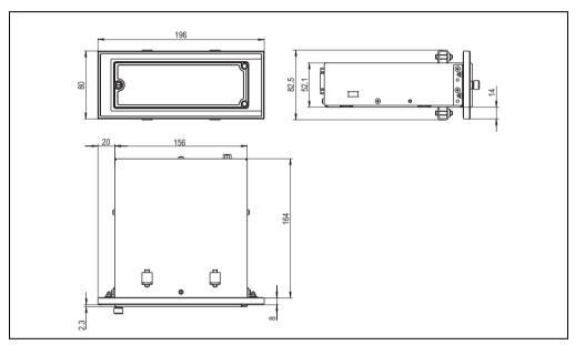
Figure 275: Dimensions - 5A5003.07 with front cover 5A5003.03
