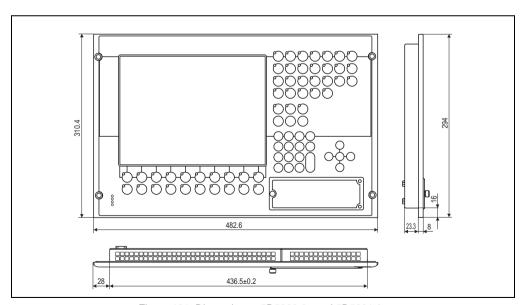
Figure 181: Dimensions - 5D5600.0x and 5D5601.0x
