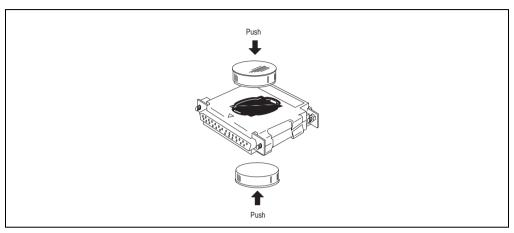
Figure 299: Hardware security key parallel adapter
