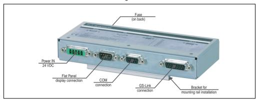
Figure 294: Remote display adapter - local unit 5A5010.01 - connections
