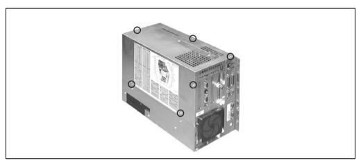
Figure 49: Opening the housing
