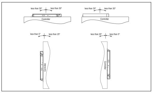
Figure 293: Mounting instructions - add-on CD-RW (revision D0 and later) with controller
