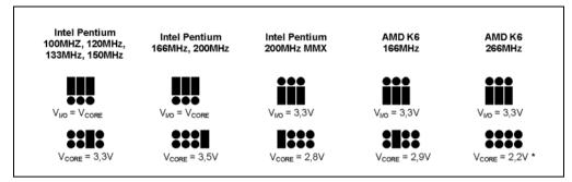
Figure 59: Setting the processor power supply voltage (jumper 2)
