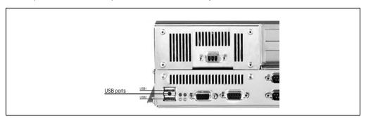
Figure 61: USB ports (5C5001.01, 5C5001.03 and 5C5601.01)
