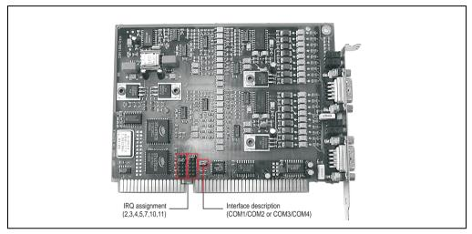
Figure 262: Jumper position
