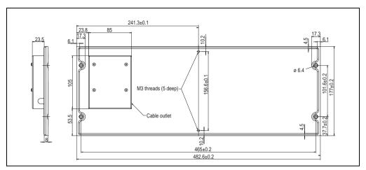
Figure 301: Installation dimensions - 19" AT keyboard (figure overleaf)
