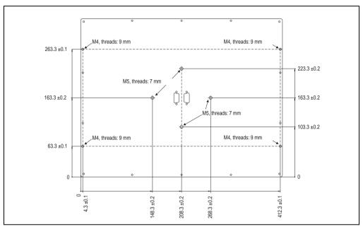
Figure 161: Flange drill holes - 5D5212.04 revision J0 and later
