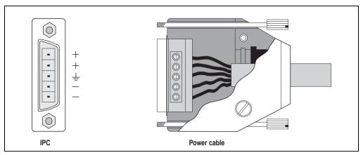
Figure 85: Plug and socket (5-pin) for DC supply
