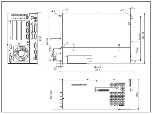
Figure 14: Dimensions - IPC5600 (5 slot design)
