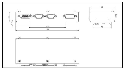
Figure 295: Dimensions - remote display adapter - local unit 5A5010.01
