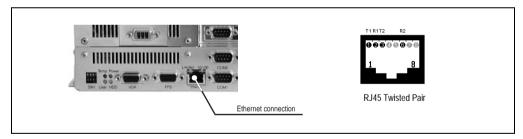
Figure 81: Ethernet connection
