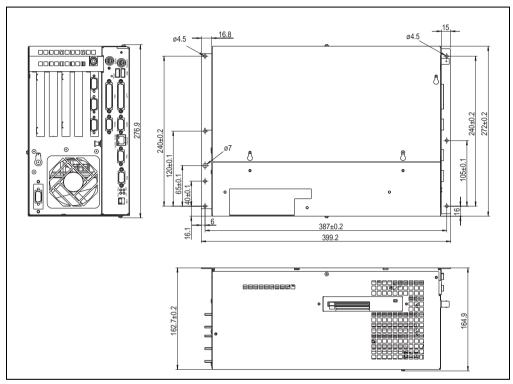
Figure 15: Dimensions - IPC5600C (5 slot design)
