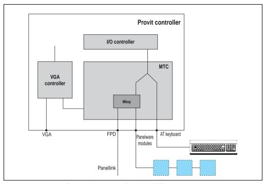
Figure 67: Maintenance Controller (MTC) block diagram
