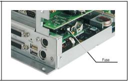
Figure 72: Fuse position for IPC5000C (left) and IPC5600C (right)
