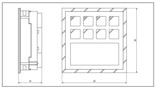
Figure 191: Dimensions - keypad module with 8 keys
