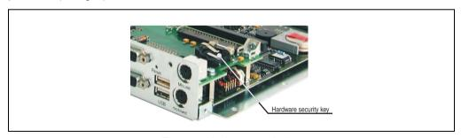
Figure 73: Hardware security key
