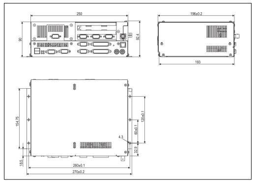
Figure 4: Dimensions - IPC5000 (2 slot design)
