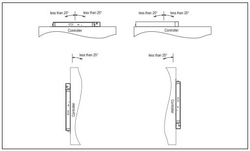
Figure 288: Mounting instructions - add-on CD ROM with controller
