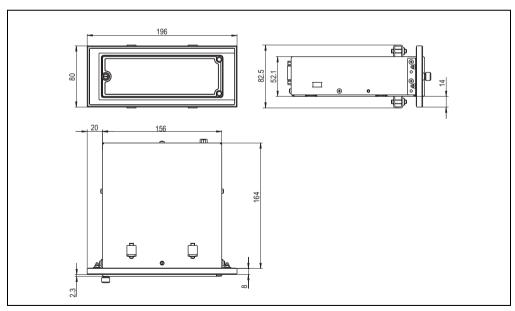
Figure 271: Dimensions - 5A5003.02 with front cover 5A5003.03
