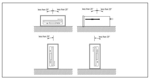
Figure 268: Mounting guidelines - external 3.5" FDD
