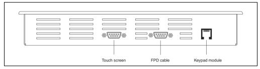
Figure 126: Connections - 5D5200.01 and 5D5210.01 revision <G0
