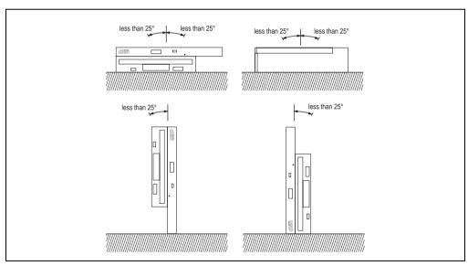
Figure 33: Mounting guidelines - 5A5600.02 controller
