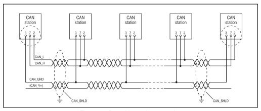
Figure 101: Bus cable - station connection
