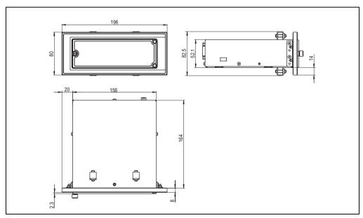
Figure 280: Dimensions - 5A5003.08 with 5A5003.03
