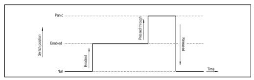
Figure 28: Enable switch - position panic
