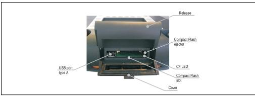
Figure 9: Compact Flash and USB slot
