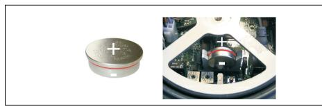
Figure 16: Inserted lithium battery
