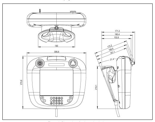
Figure 3: Dimensions for the entire device
