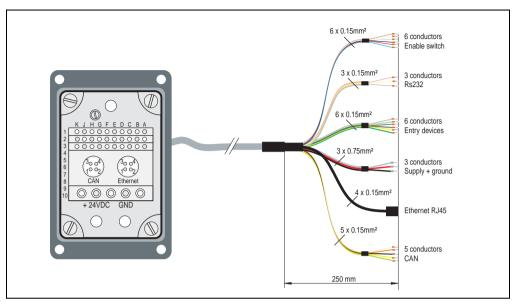
Figure 38: Cable layout for the switching cabinet cable
