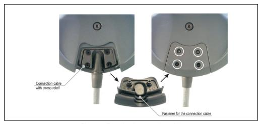
Figure 30: Fastening the connection cable
