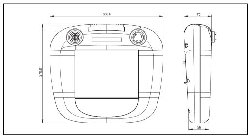
Figure 5: Operating unit dimensions
