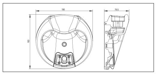
Figure 24: Dimensions for the handle
