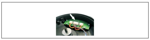
Figure 69: Connecting the enable switch connector (ST1)
