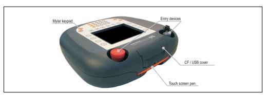
Figure 4: Mobile Panel operating unit
