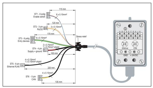
Figure 33: Connection cable specifications
