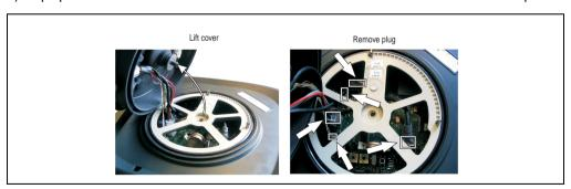
Figure 65: Removing the attachment cable
