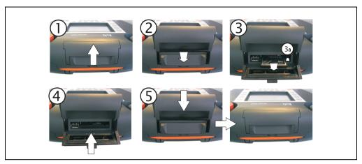
Figure 11: Removing a Compact Flash Card
