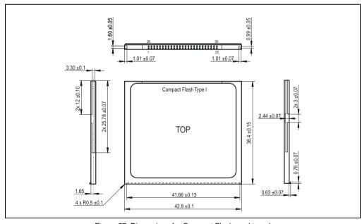
Figure 57: Dimensions for Compact Flash card type I
