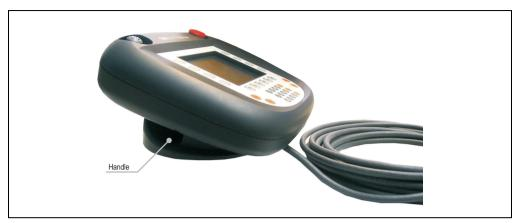
Figure 22: Operating unit, handle and connection cable
