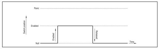
Figure 27: Enable switch - position enable
