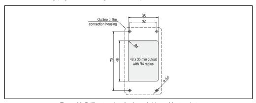
Figure 36: Drilling template for the switching cabinet socket
