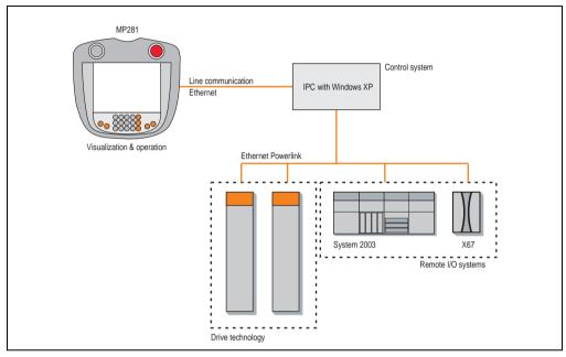
Figure 53: Mobile Panel as a thin client
