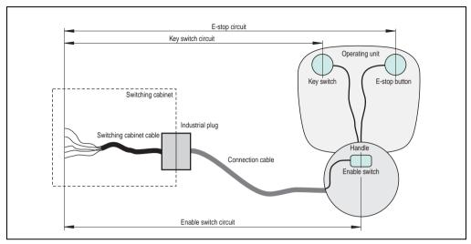
Figure 47: Current load of the enable switch and entry device circuit
