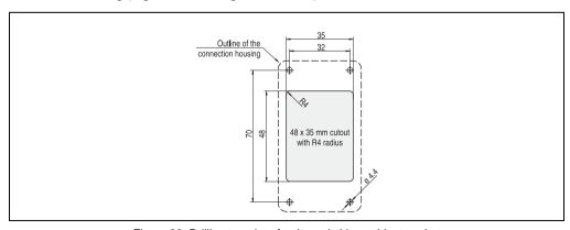
Figure 39: Drilling template for the switching cabinet socket
