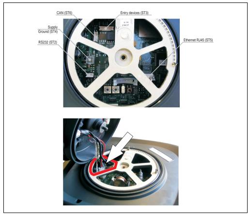
Figure 70: Connectors and cable arrangement
