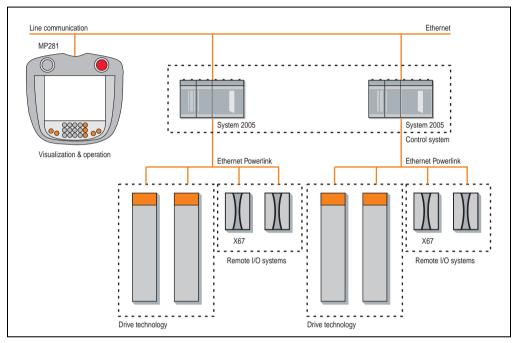
Figure 50: Operation and monitoring with the Mobile Panel
