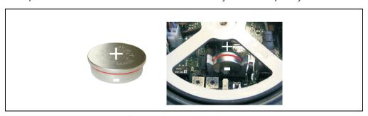
Figure 76: Inserted lithium battery
