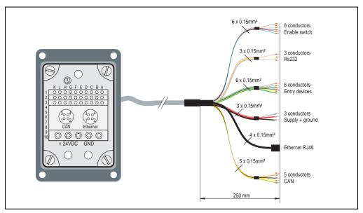
Figure 35: Cable layout for the switching cabinet cable
