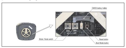
Figure 15: Back of the operating unit - switches, buttons and batteries
