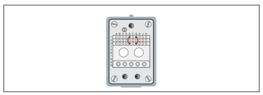
Figure 42: Cable layout for the strapping plug
