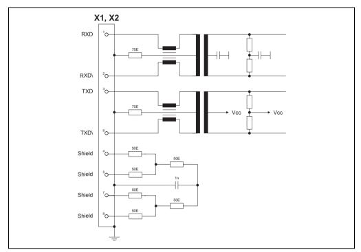
Figure 49: Input/Output Circuit Diagram AC112
