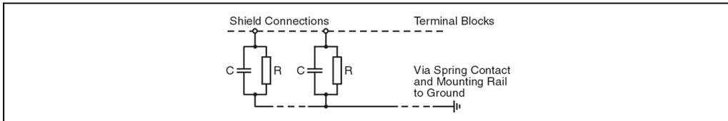
Figure 167: AT660 shielded connection
