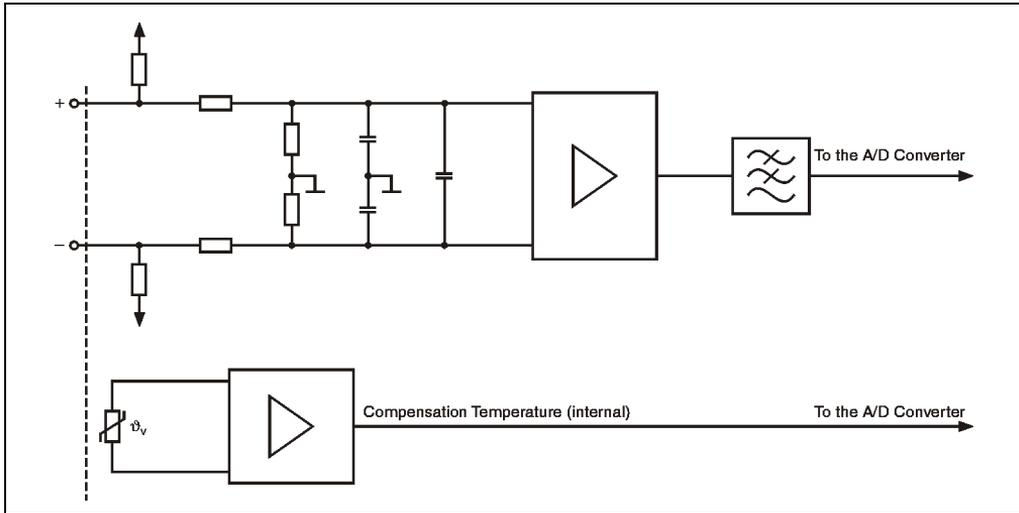
Figure 168: AT660 input circuit diagram
