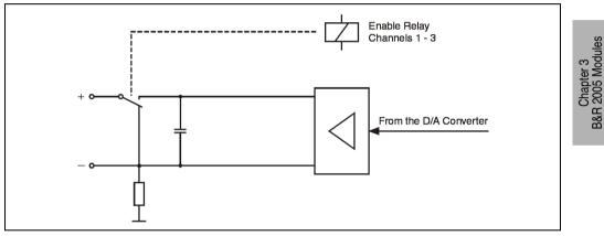
Figure 156: AM055 output circuit diagram
