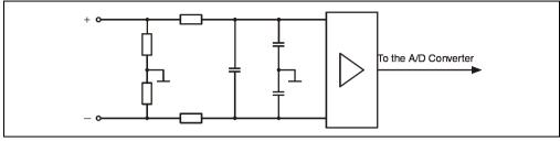
Figure 155: AM055 input circuit diagram
