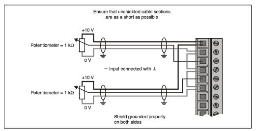
Figure 154: AM055 potentiometer operation
