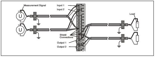
Figure 153: AM055 signal cable connection
