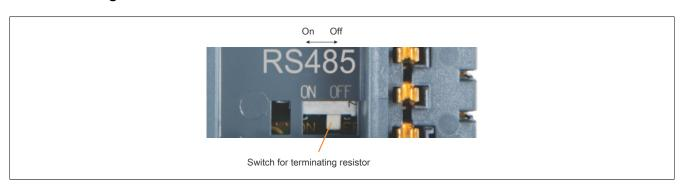
A terminating resistor for the RS485 interface is already integrated on the bus base. The terminating resistor is switched on or off with a switch. An enabled terminating resistor is indicated on the power supply module by LED "T".
